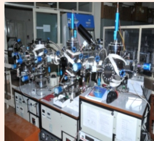
A specially designed multi chamber PLD and dc/rf-magnetron sputtering coupled in series
