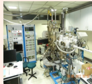
Plasma Assisted Molecular Beam Epitaxy Machine (PAMBE), RIBER Compact 21E,
