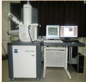
Field Emission Scanning Electron Microscope (Make: Zeiss; Model: Supra 40VP)
