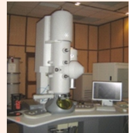
High Resolution Transmission Electron Microscope (Make: Tecnai G2 F30 STWIN)
