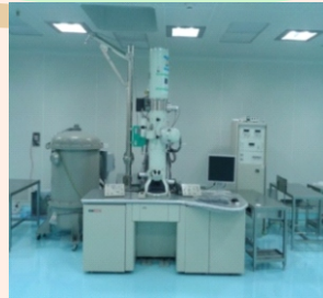
High Resolution Transmission Electron Microscope (Make: JEOL: JEM - 2100F)
