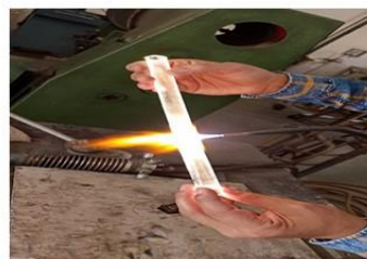
Vacuum sealing in quartz tube
