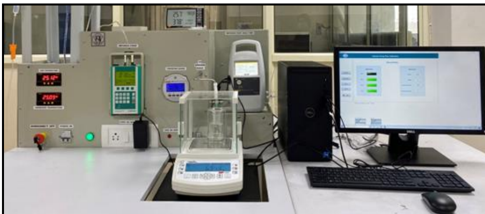
Set up for calibration of Infusion Pump Analyzer
