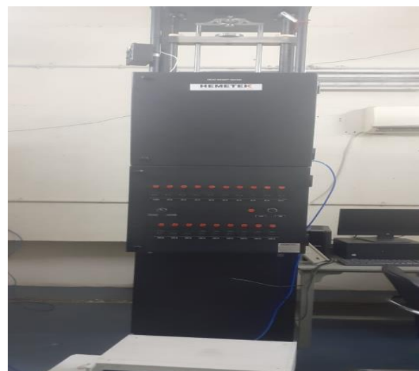
5 kN fully automatic dead weight force machine established at Force Metrology
