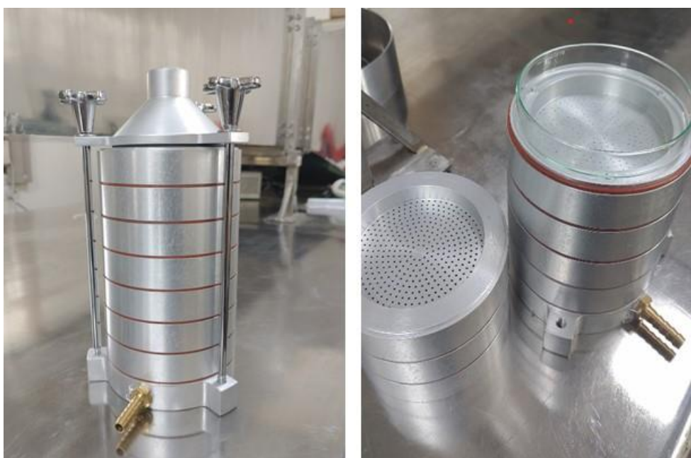
Designed and developed bio-aerosol sampler
