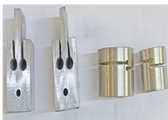
Fabrication of Hole Plates (Mild Steel)
