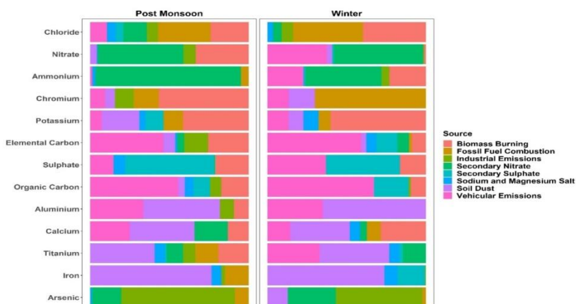
Percentage contribution of different species and sources to total PM 2.5 for winter and post-monsoon seasons in Delhi (Source: Joshi et al (2022); Environmental Science & Technology , doi:10.1021/acs.est.1c06864)
