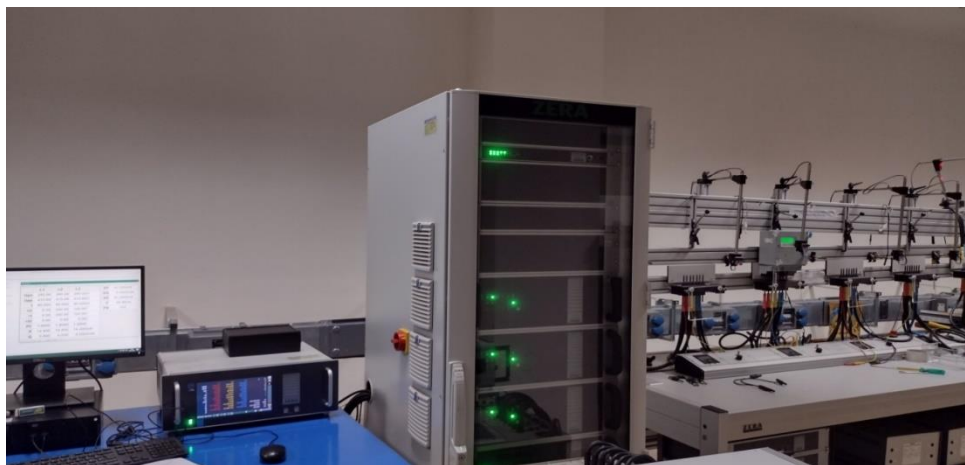
Compliance Testing of smart energy meter using multi-position meter test system
