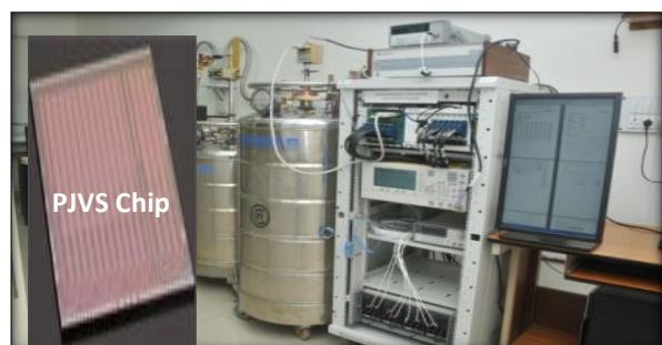
Established PJVS system at CSIR-NPL India for quantum DC voltage metrology
