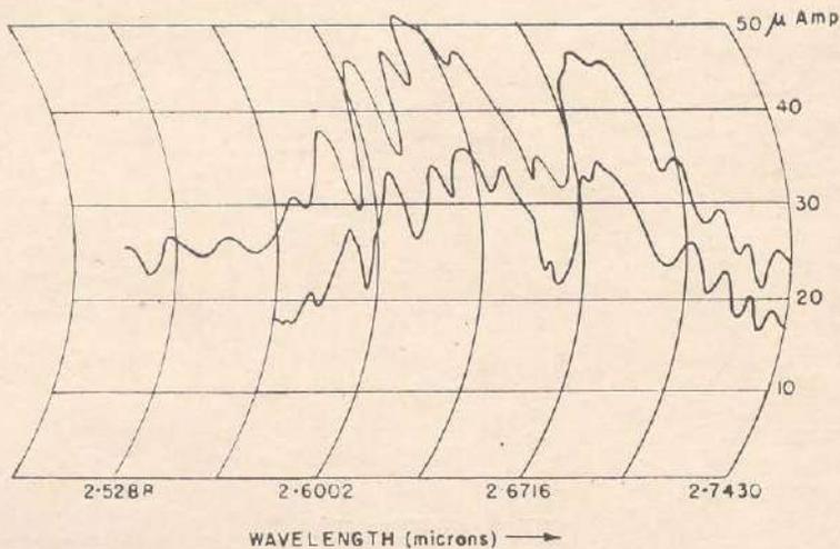
**Fig. 22. Atmospheric water vapour bands between 2.52 and 2.74 microns taken with the instrument on an Esterline Angus Recorder. Two curves represent two repetitions.**
