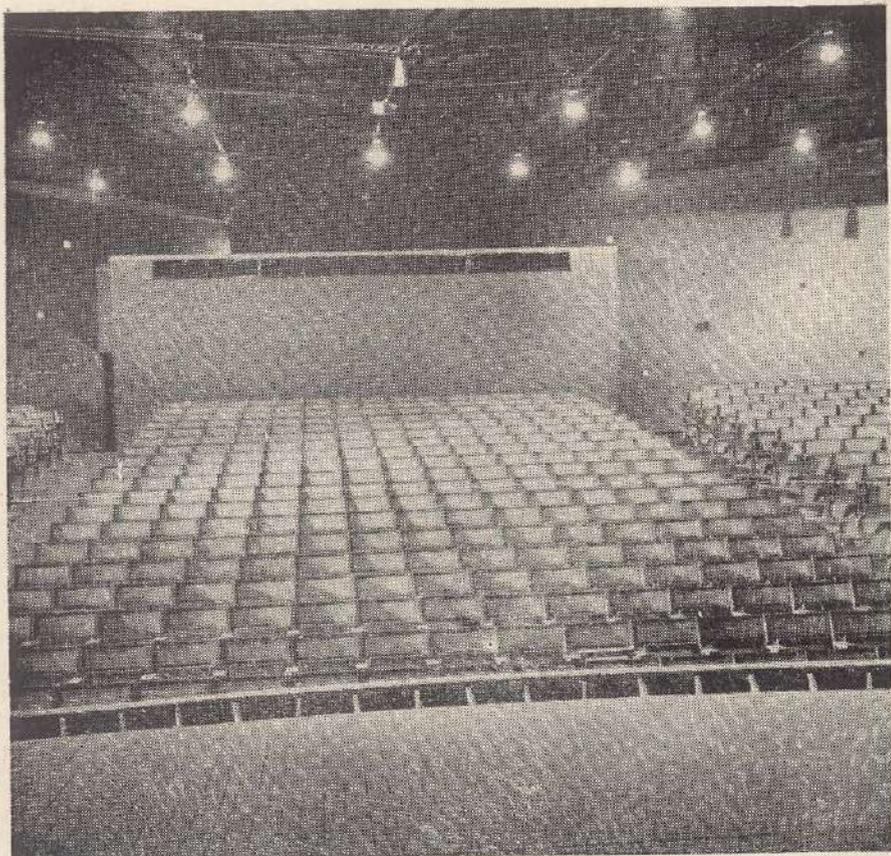
**Fig. 6.** Inside view of the Tagore Theatre Chandigarh from stage showing raked seats, resonators in back partition and exposed trusses in the ceiling.
