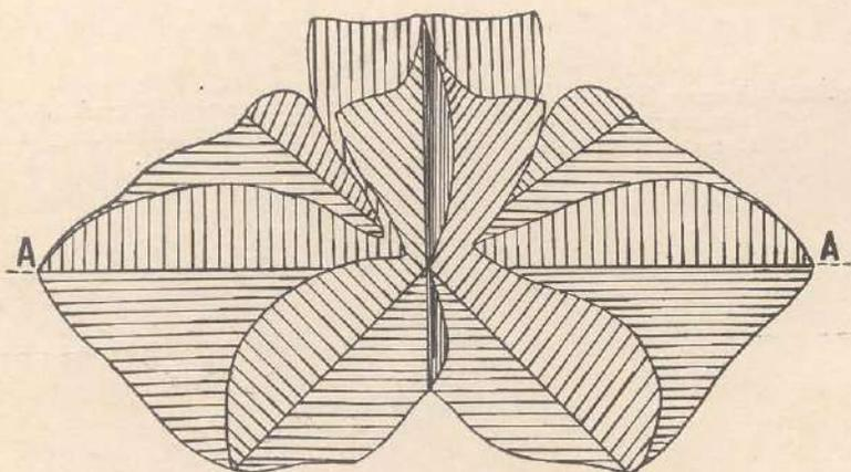
Fig. 24. Directionality Patterns of Sound Radiation from a Siren
