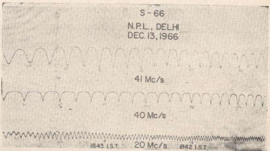
Fig. 14. Faraday Fading Record of Satellite Transmissions.
