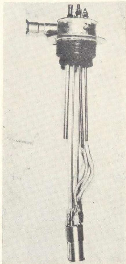
Fig 7 12 kOe superconducting magnet developed and fabricated at the Laboratory.
