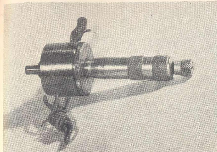
Fig 10 Piezoelectric micrometer developed at the Laboratory. The body to be displaced is mounted at the tip of the micrometer. The coarse movement upto a distance of 10 mm can be provided through the micrometer screw head, while the fine displacement in the range 0.025  $\mu$ m to 15  $\mu$ m may be made by applying suitable DC voltage across the two terminals.
