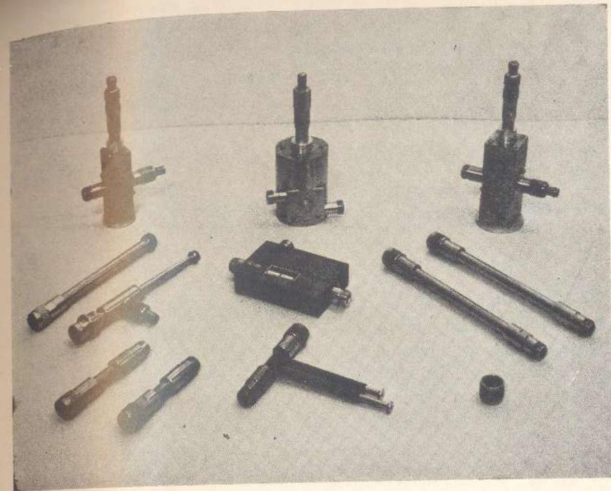
Fig 13 Coaxial line components developed at the Laboratory. Left to Right, Top row : Coaxial frequency meters (6.5 GHz to 10.2 GHz, and 2.5 GHz to 6.5 GHz). Middle row : Coaxial terminator (2.0 GHz to 12.4 GHz), Tunable probe (3.95 GHz to 12.4 GHz), 10 db Directional coupler, Coaxial attenuators (3.0 GHz to 12.4 GHz). Bottom row : Fixed attenuators (6.0 GHz to 12.4 GHz), Double-stub tuner, Fixed short circuit.
