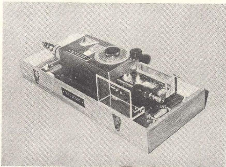
Fig 2 30 MHz Waveguide Below Cut-Off Standard attenuator.
