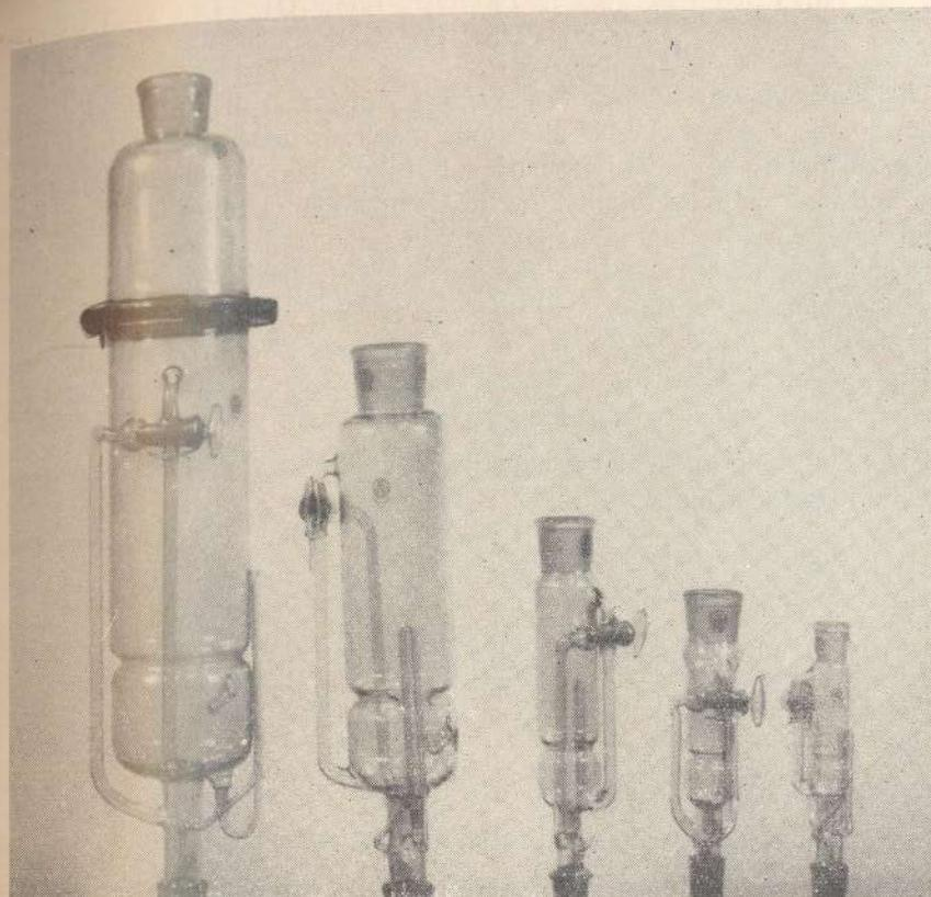
Fig 16 Multipurpose solvent extractor developed and fabricated at the Laboratory in different capacity ranges varying from 20 ml to 2l. It is useful in preparation and purification of fine chemicals ; analytical determination ; industrial, agricultural and bio-chemical diagnostic aid ; environmental pollution ; research and academic pursuit ; and standardization.
