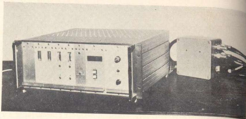
Fig 11 140 MHz ATS-6 radio receiving system designed jointly by the NPL and the Max Planck Institute, West Germany, under a collaborative programme with that Institute, and fabricated at that Institute. The system started recording both the amplitude and the phase of the radio beacon transmissions for the ATS-6 satellite from 1 August 1975 at the NPL, New Delhi, and later operated at the Gauhati University also.
