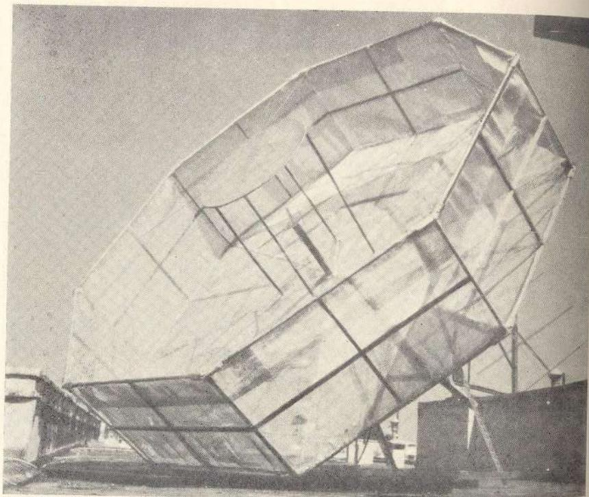
Fig 12 Short back-fire antenna for 140 MHz, designed and installed at the Laboratory for observation of the ionospheric effects on the signals transmitted by the ATS-6 satellite.
