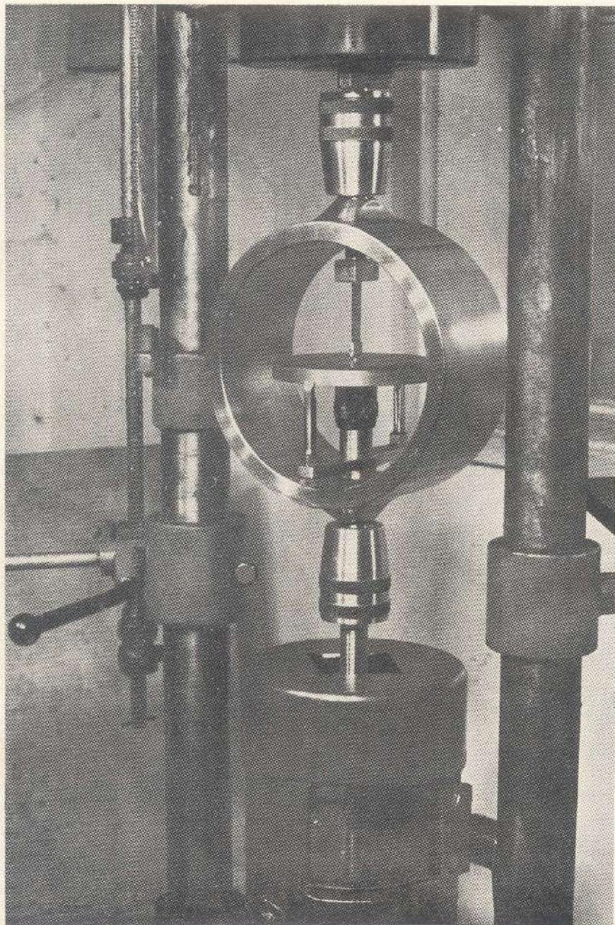
Fig 3 Verification of a universal testing machine using a calibrated proving ring.
