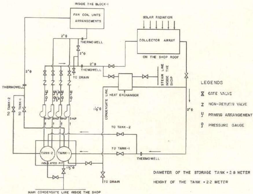
Fig 8 Design of the solar space heating system for the Hardwar factory of the Bharat Heavy Electricals Ltd.
