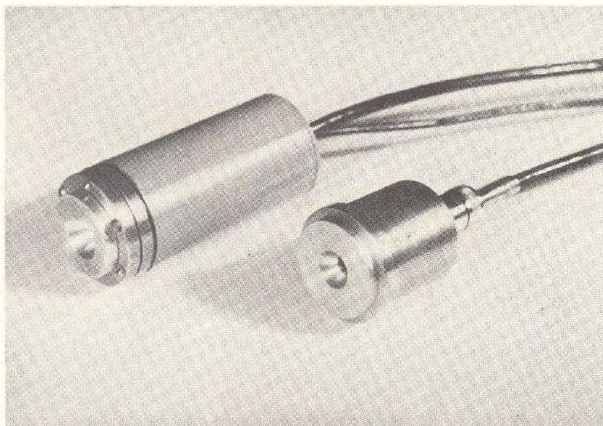
Fig 4 Two models of pyroelectric infrared detector assemblies developed and fabricated at the Laboratory. The preamplifiers are enclosed within the assemblies. These detectors, with a noise equivalent power (NEP) of  $7.5 \times 10^{-8} \text{ W/Hz}^{1/2}$ , find a variety of applications in fast detection of radiant energy.
