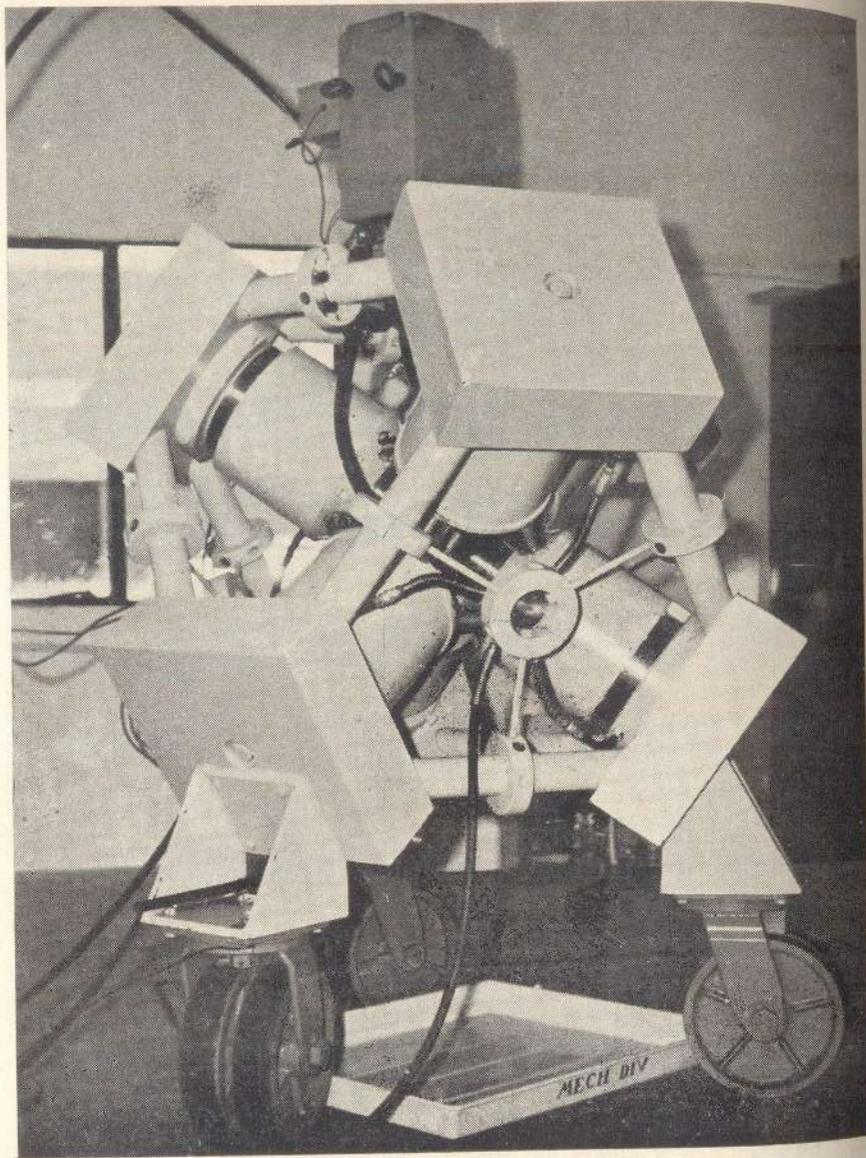
Fig 14 The 200-ton cubic press used for laboratory-scale production of industrial grade diamonds in various shapes and sizes. The material producing the diamonds is taken in a cubic form, and is subjected to uniformly high pressure under controlled high temperature to make diamonds.
