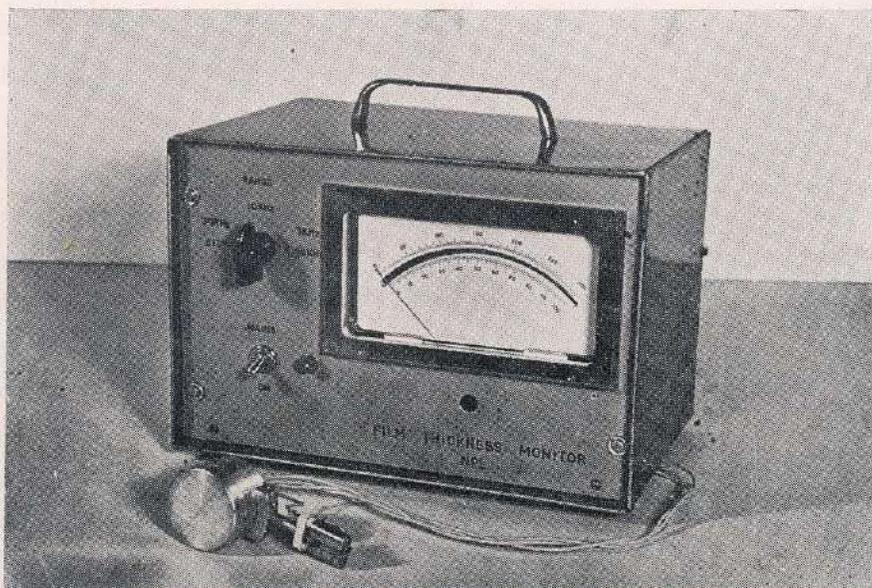
**Fig 9** Electronic monitor for vacuum deposited thin films, designed and developed at the Laboratory.
