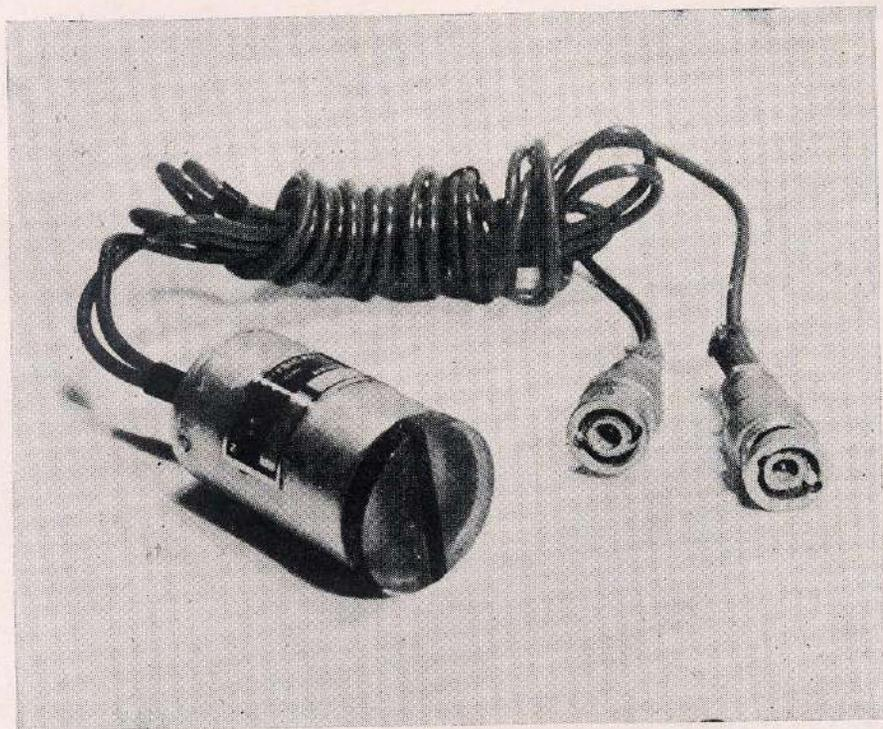
**Fig 11 Twin normal probe (dead zone 2—6 mm) for ultrasonic non-destructive testing and thickness gauging, developed at the Laboratory.**
