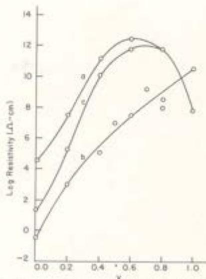
Fig. 2: Variation of Log resistivity Vs  $x$  for (a) Screen printed and sintered film of  $Zn_x Cd_{1-x}S$ . (b) Vacuum evaporated  $Zn_x Cd_{1-x}S$  thin film (c) Film (a) annealed in  $H_2$  atm at  $200^\circ C$  for 30 min.
