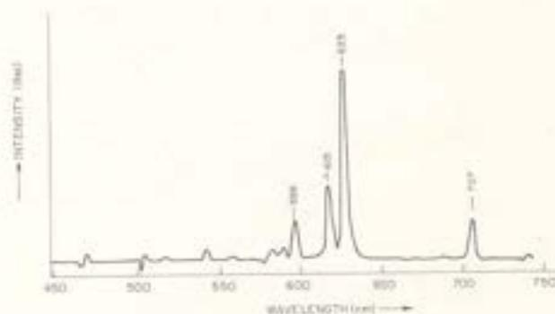
Fig. 3 Emission Spectrum of  $Y_2O_3:S:Eu$  Under UV Excitation (365 nm).
