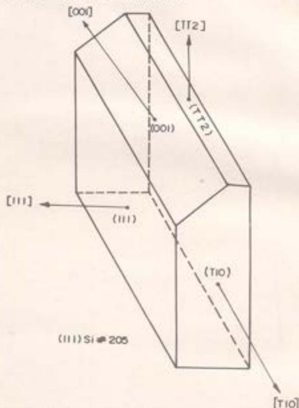
Sketch of a specimen crystal block prepared with surfaces along the following lattice planes: (111),  $(\bar{1}\bar{1}0)$ , (001) and  $(\bar{1}\bar{1}2)$ . With this specimen DXS measurements could be made in eight planar sections of the reciprocal space around four different reciprocal lattice points.
