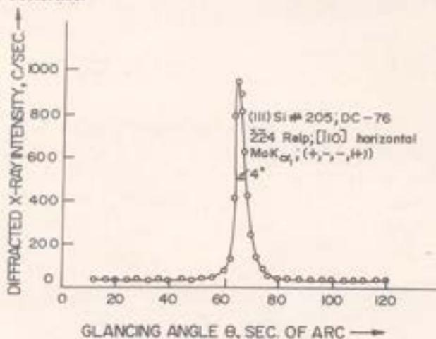
A typical diffraction curve of the silicon single crystal block recorded with  $\bar{2}\bar{2}4$  diffracting planes in symmetrical Bragg geometry using  $MoK_{\alpha 1}$  radiation. It has a half width of only 4 sec of arc.
