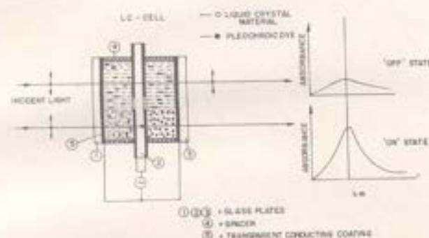
Fig. 5 Basic Construction of a Positive Contrast Colour Display without Polarizers
