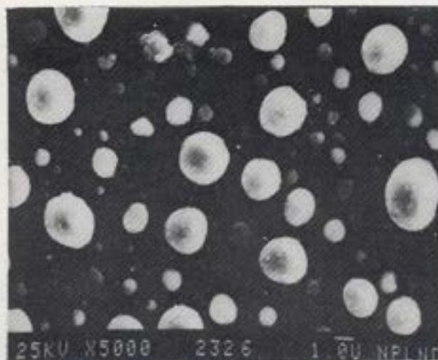
SEM micrograph of thermally evaporated silver film annealed in air at  $400^\circ\text{C}$  showing agglomeration
