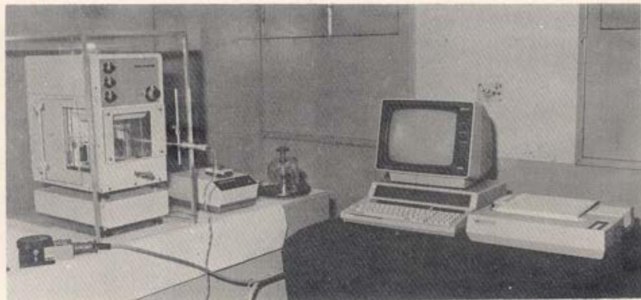
1 Kg Mass Comparator with computer controlled weight handler
