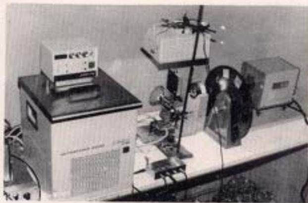
Fig. 1: Spectral Responsivity Measurement Apparatus.
