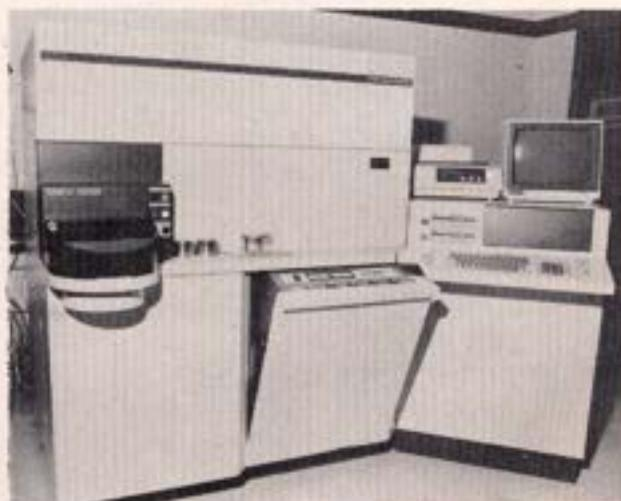
Rigaku X-ray Fluorescence Spectrometer-3070 E
