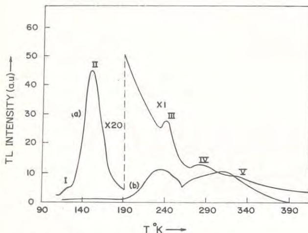
Fig. Glow curves of the  $Gd_2O_2S:Tb$  phosphor, (a) original (b) after  $H_2S$  firing.
