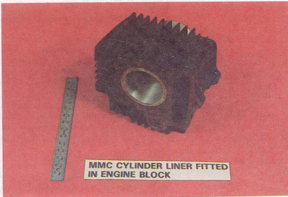
Fig. 1 MMC circular tube fitted as liner in cast iron engine block
