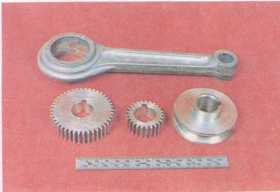
Fig. 2 Some of the secondary processed MMC components
