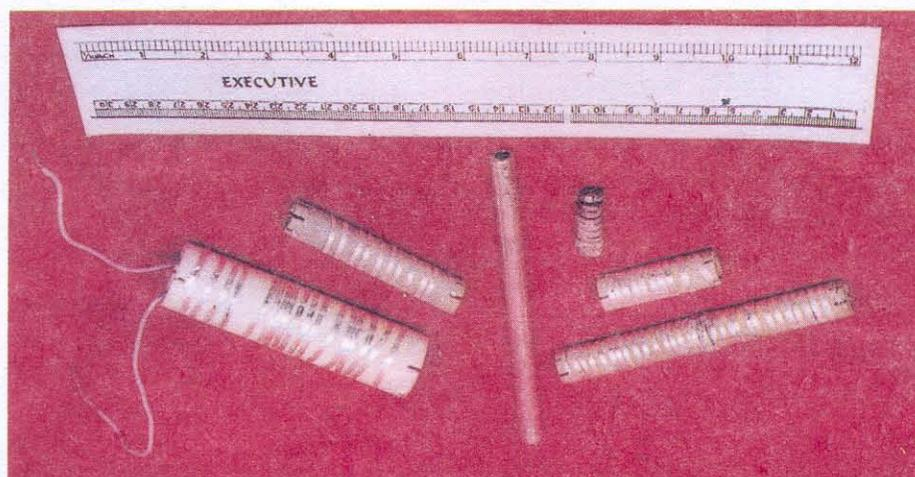
Photograph showing some of the superconducting coils of different lengths, (up to 5 m) of silver clad HTSC BPSCCO tapes.
