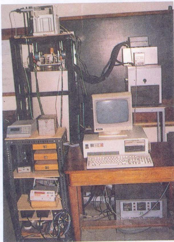
Automatic Computer based solid density standard system
