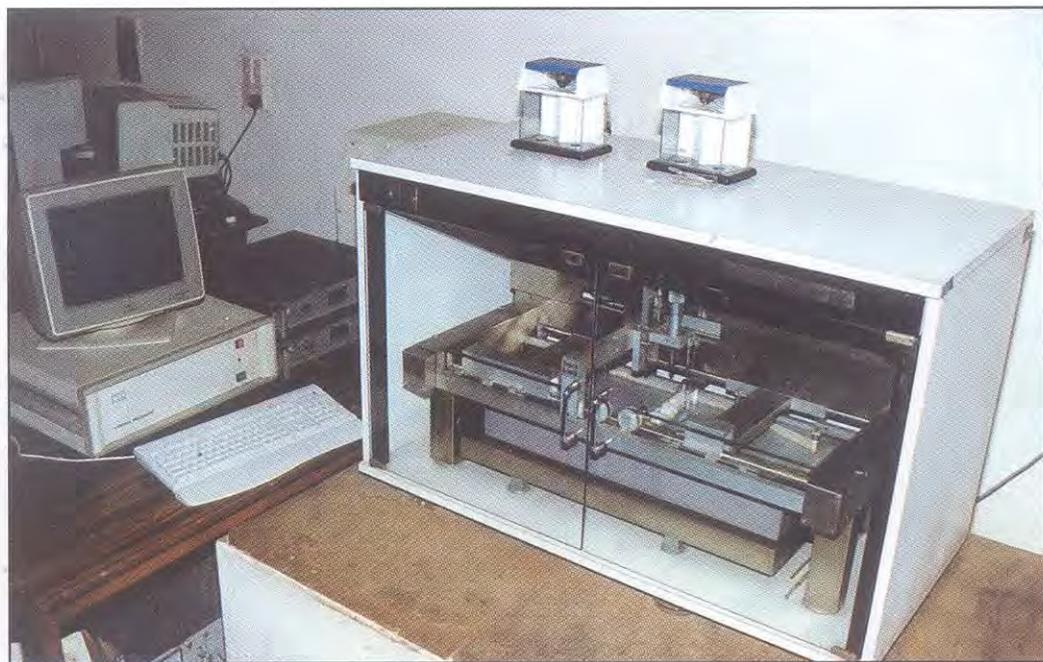
Fig. 5.7 : Langmuir - Blodgett film deposition system for fabrication of molecular mono/multilayers
