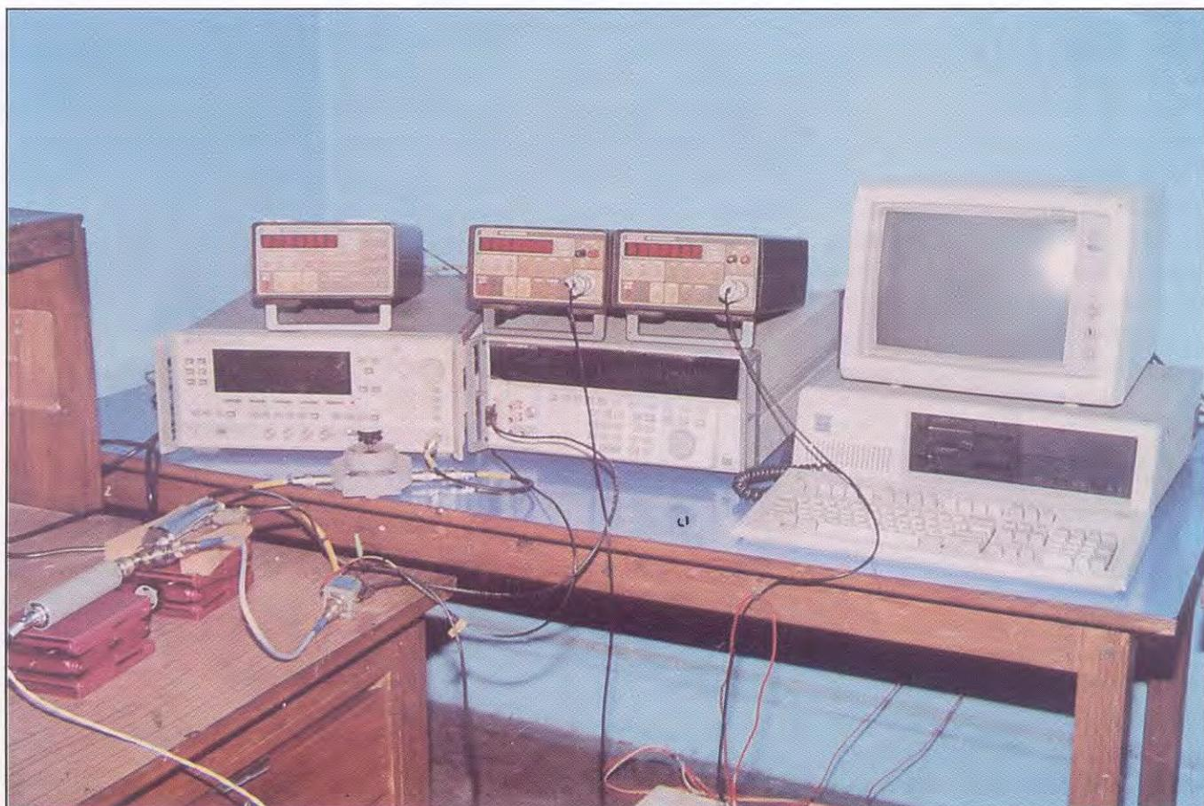
Fig. 2.3 : Setup for Intercomparison of HF Voltage Transfer Standards
