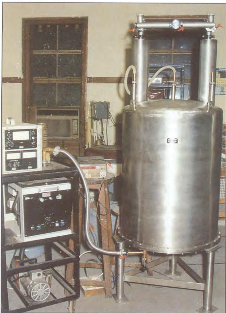
**Fig. 9.3 :** The liquid helium cryostat housing the 2.35 T Superconducting magnet. The cryostat has a 52 mm room temperature bore, 1.35 l pr day L-helium evaporation and a refill time of 90 days.
