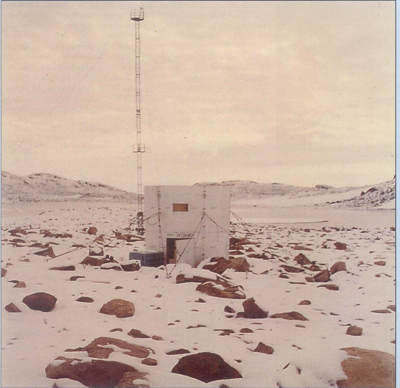
Fig. 7.1 : Monostatic acoustic sounder and 28 m instrumented tower installed at "Maitri", Antarctica
