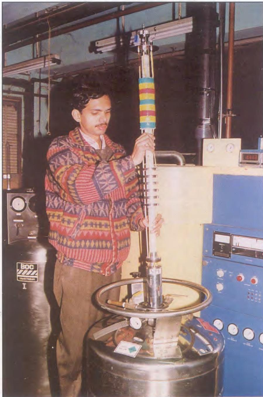
Fig. 9.5 : A 3T, 28 mm bore superconducting magnet which can be used as an insert magnet in a standard 100 litres liquid helium container.
