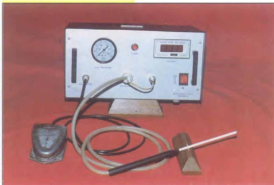
**Fig. 9.2 :** A cryosurgical unit for ENT cancer developed at NPL.
