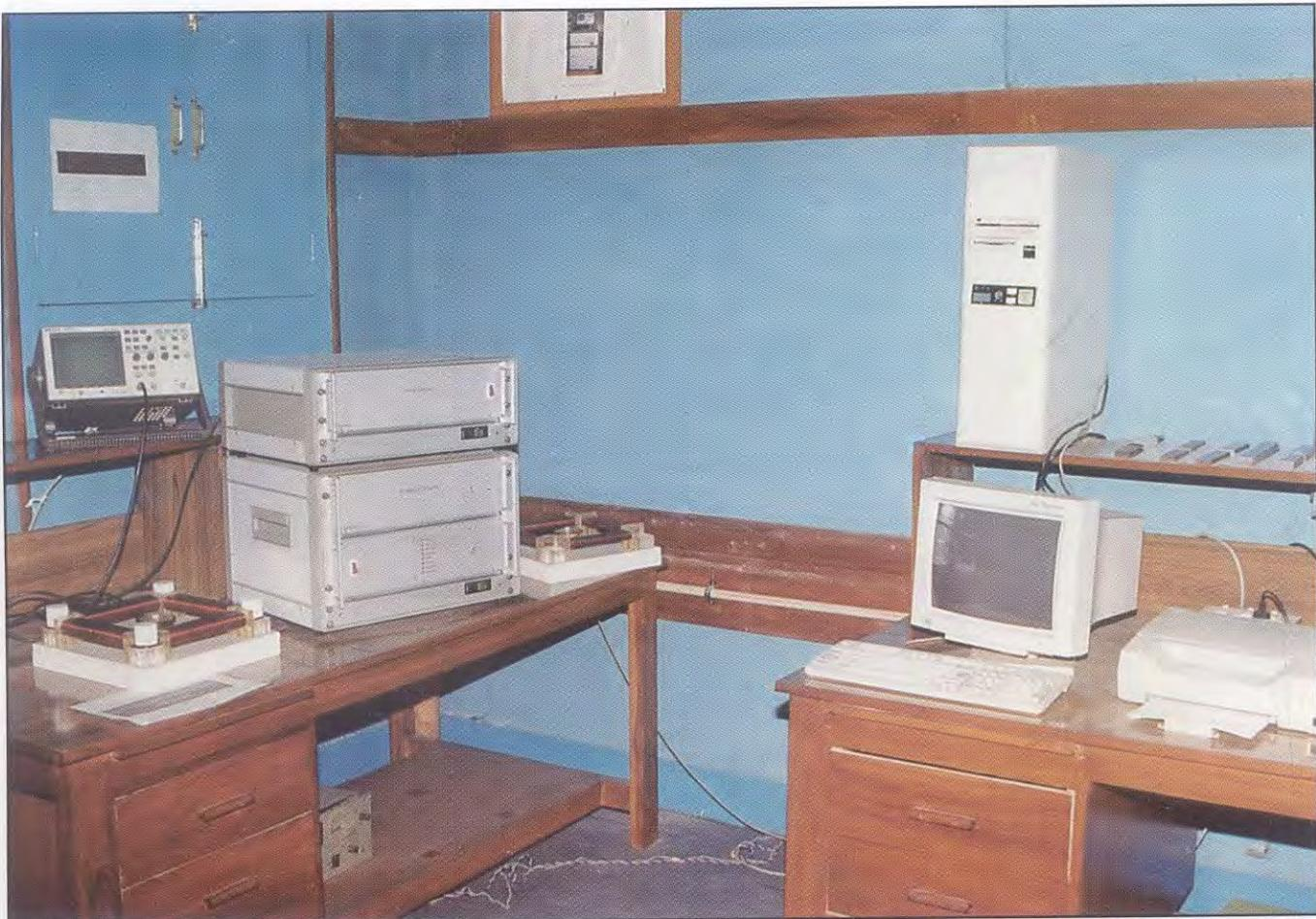
Fig. 2.5 : AC Magnetic Measurement System for Soft Magnetic Materials
