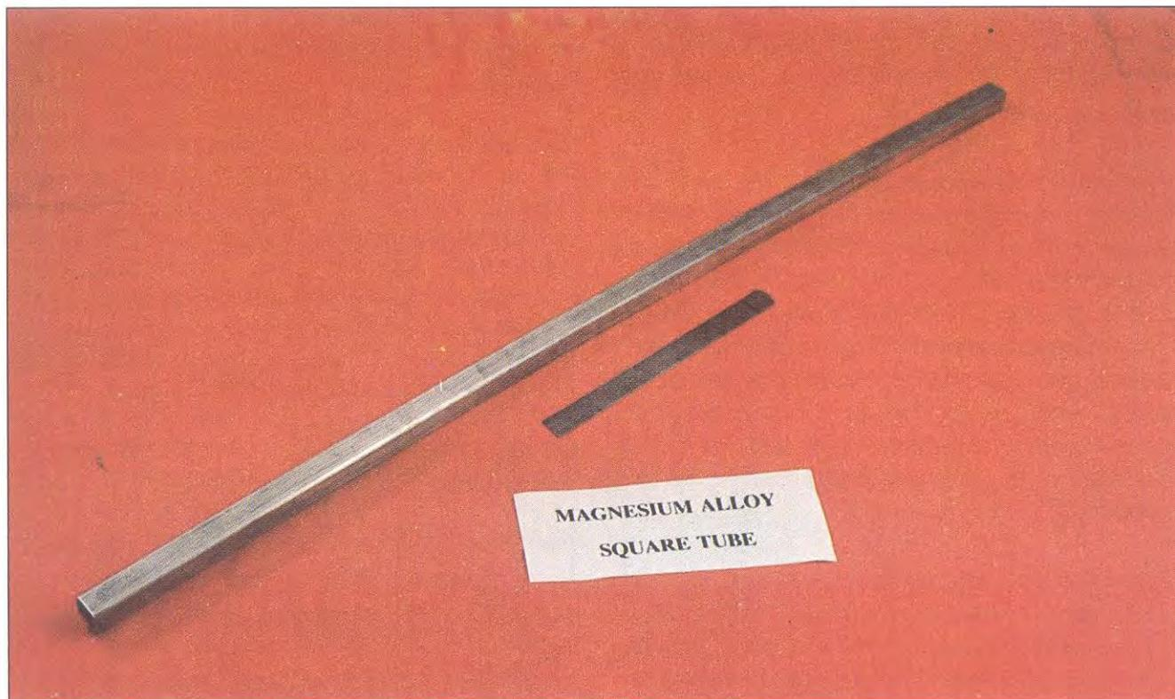
Fig. 3.1: Pictorial view of square tubes of Mg-alloy, ZK 30, developed at NPL for space applications
