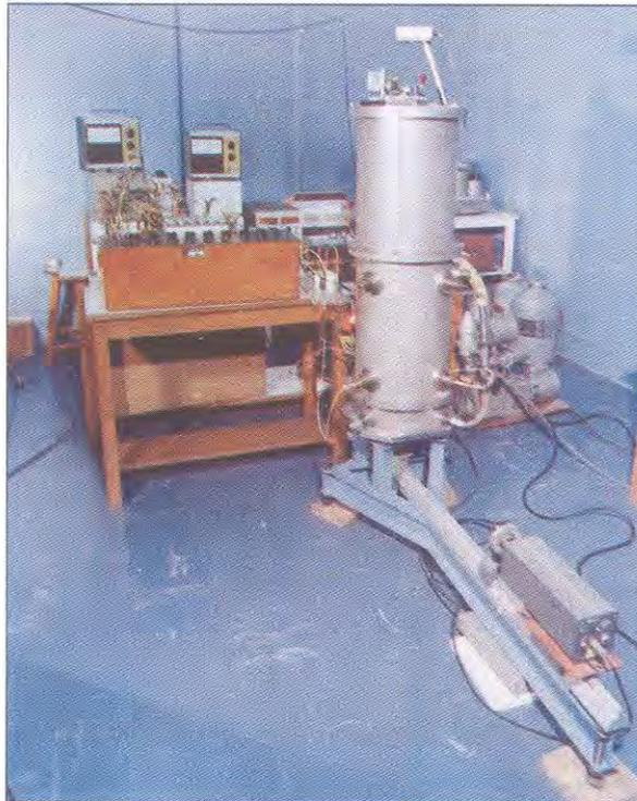
*Fig. 2.2: Calculable cross capacitor established at NPL as the 'Primary Standard' used for realisation of 'National Standards' of capacitance, resistance and inductance*
