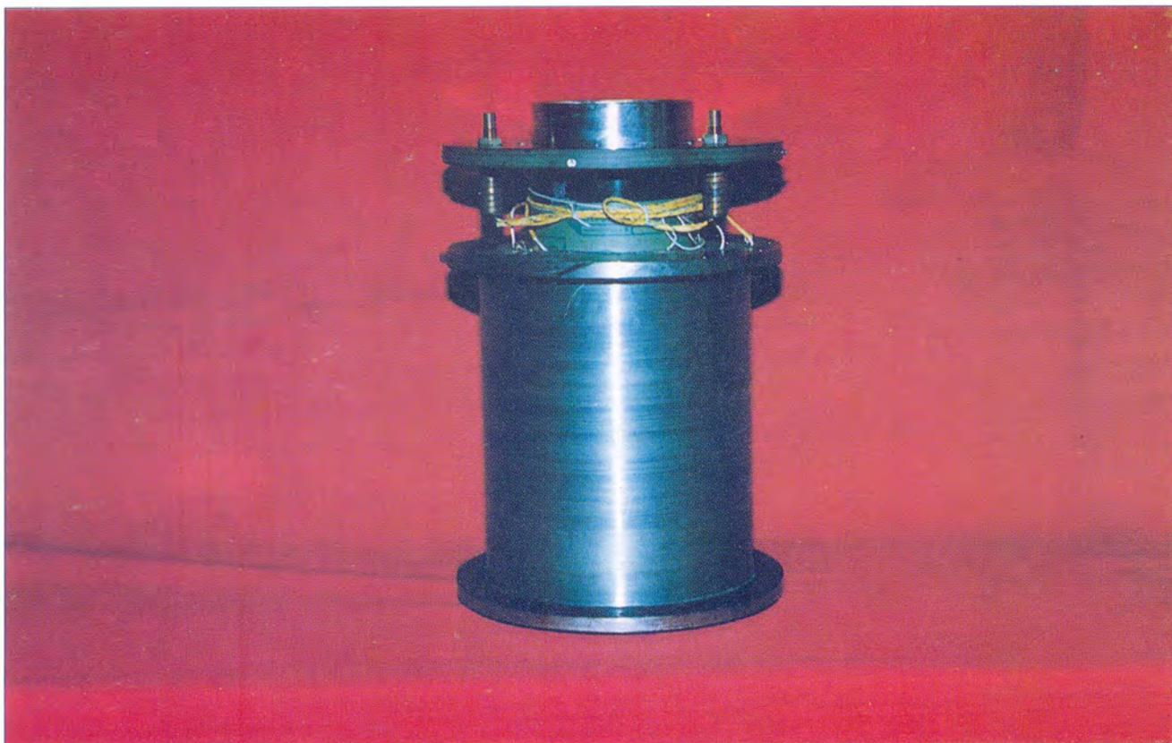
Fig. 9.2: A large bore 104 mm, 7 Tesla superconducting magnet wound with Cu/Nb-Ti conductor. The magnet will be used as a background field magnet. It will have a Cu/Nb<sub>3</sub>Sn conductor insert coil for producing a central field of 11 Tesla
