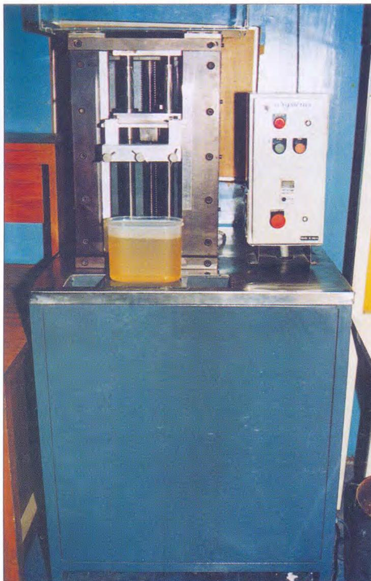
Fig. 5.9: A custom made Dip-Coating Unit installed at NPL. Substrates of dimensions up to the size 300 mm x 300 mm can be deposited using this facility.
