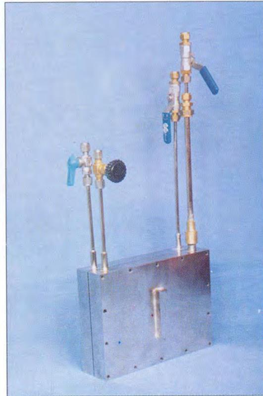
Fig.9.7: The assembled heat exchanger using
