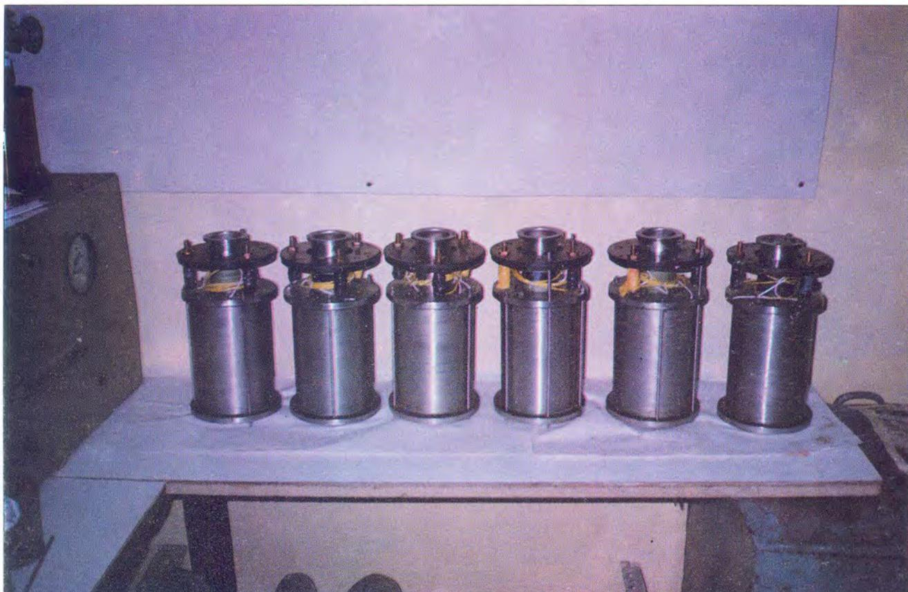
*Fig.9.1: Six units of 52 mm bore superconducting magnets designed and fabricated by NPL to produce a field of more than 7 Tesla at 100 amp*
