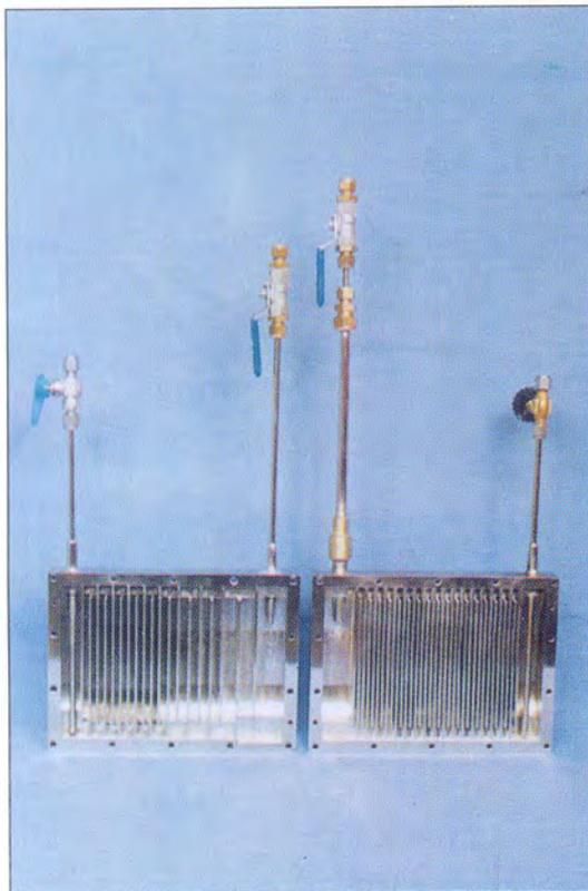
Fig.9.6: Heat exchanger (saturator), a critical part
