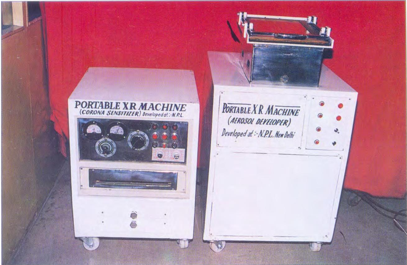
Fig. 5.19: Portable X-ray radiography machine developed by NPL
