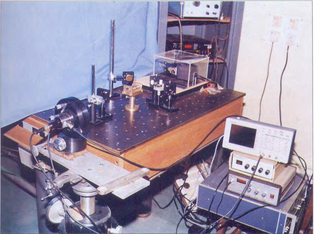
Fig. 1.3: Extended cavity diode laser with cesium saturated absorption spectrometer
