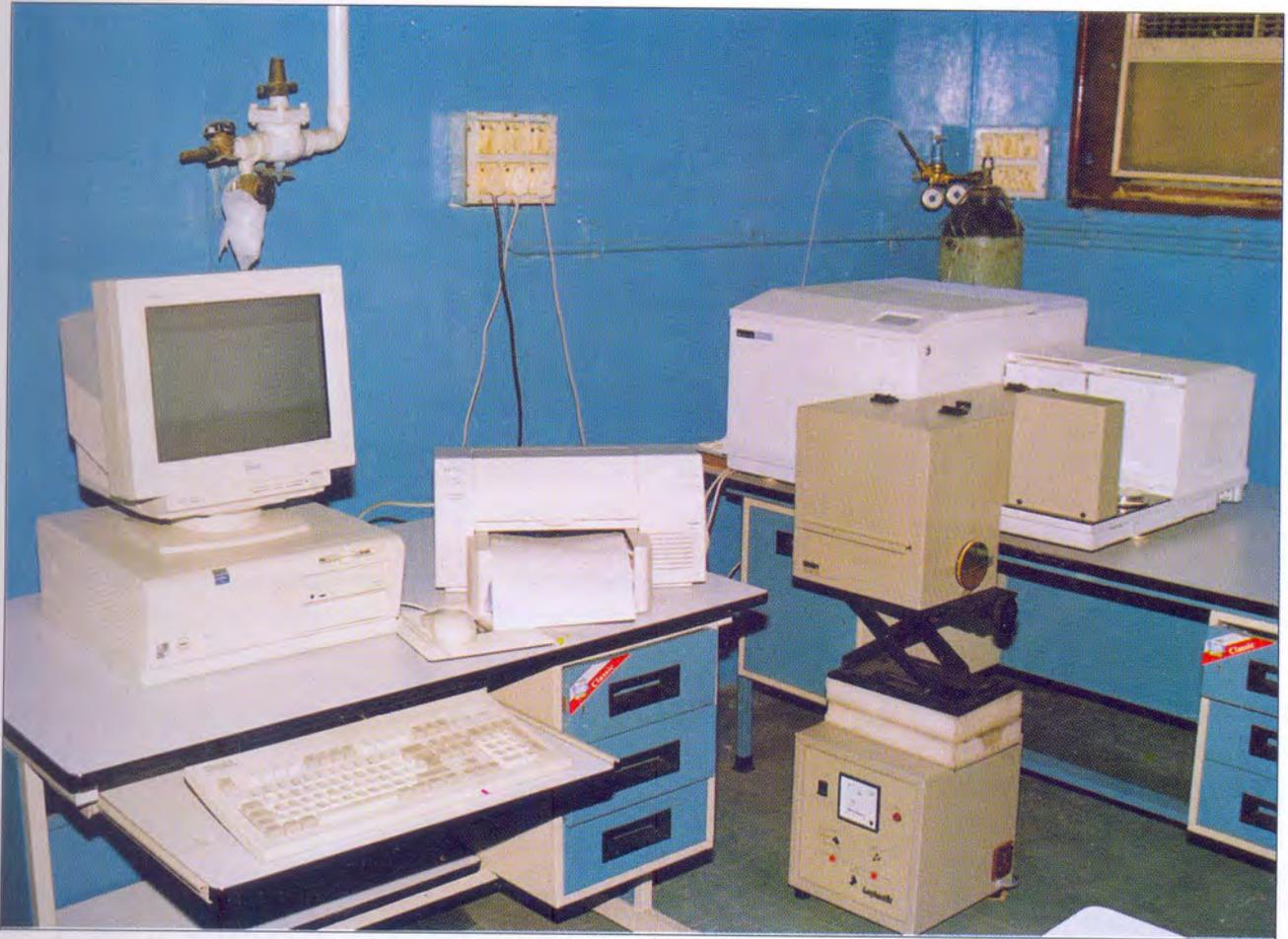
Fig. 1.6: FTIR spectrophotometer set up mounted with integrating sphere for diffuse/total-reflectance/transmittance studies in the spectral range  $2.5 \mu\text{m}$  to  $25 \mu\text{m}$
