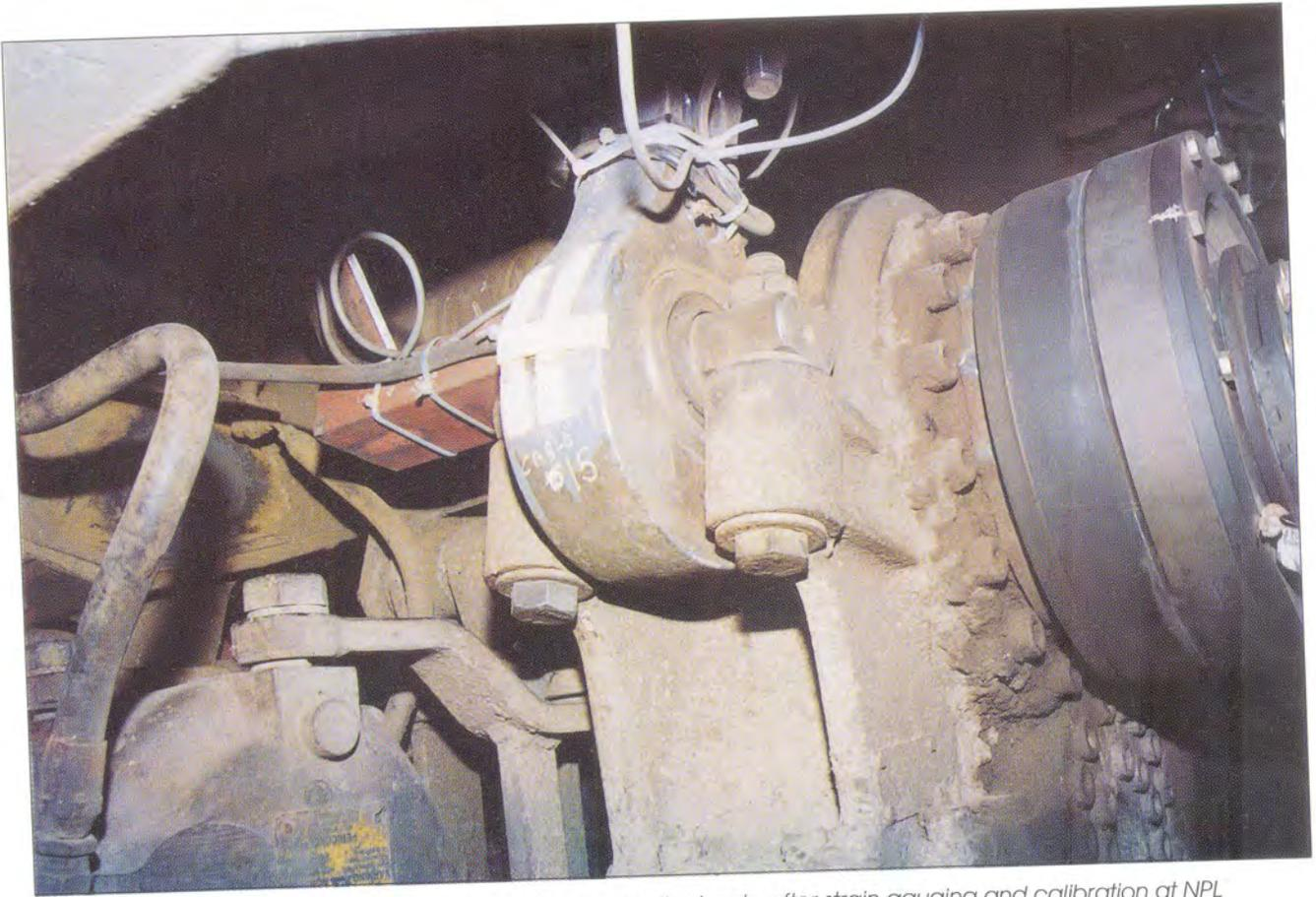
Fig. 1.4 (b): Gear box torque reaction link fixed in the bogie after strain gauging and calibration at NPL
