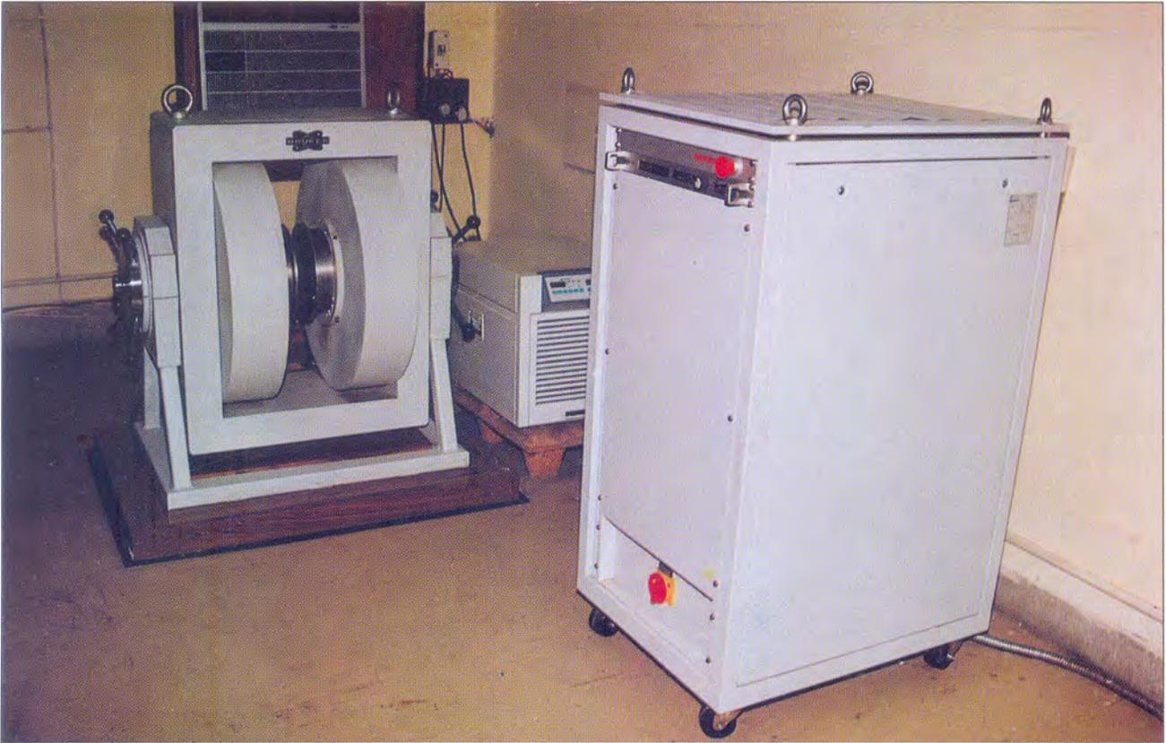
Fig. 2.4 (a): Photograph of 25 cm pole diameter electromagnet
