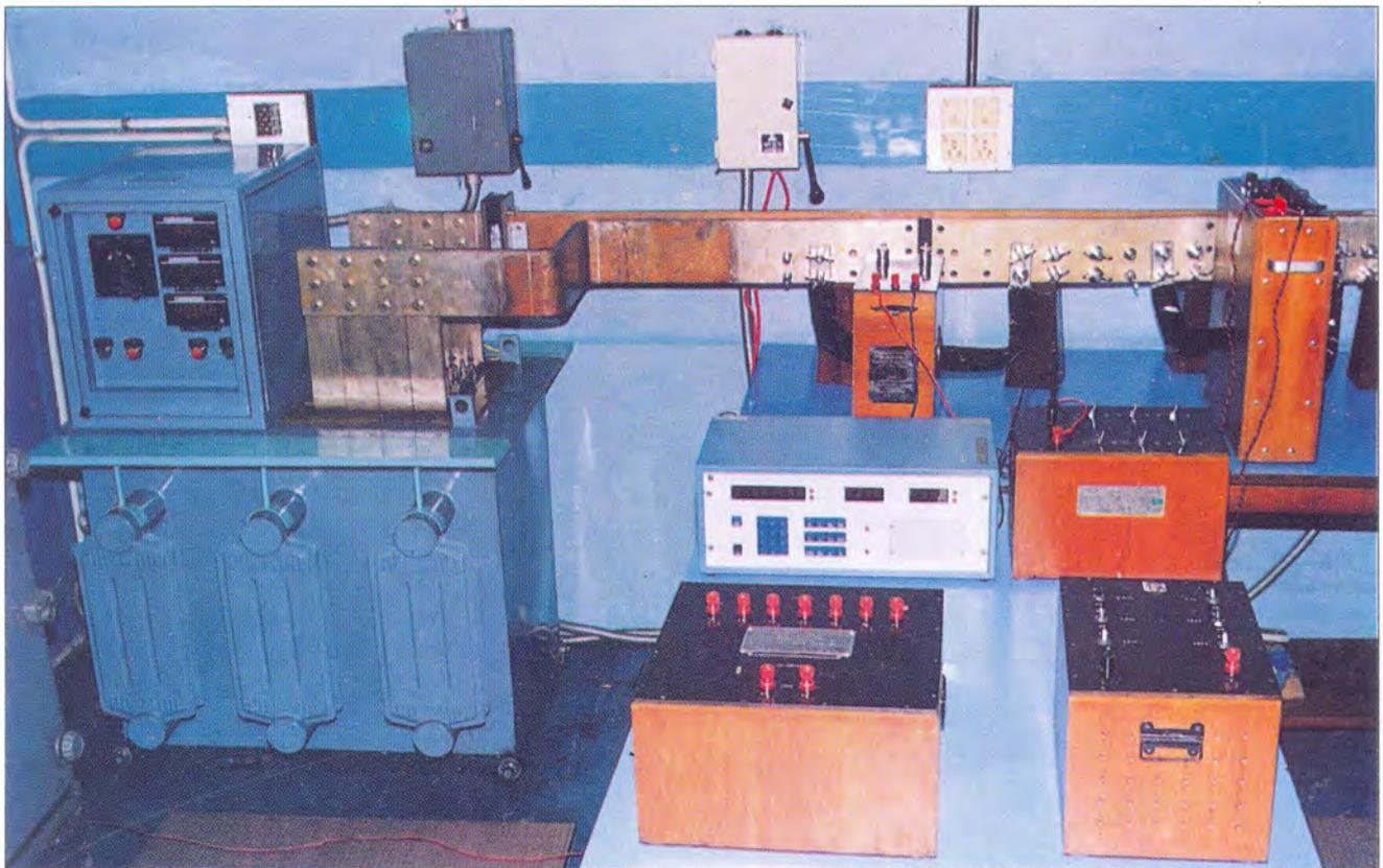
Fig. 2.2: Experimental set up for calibration of current transformers up to 5000 A/5 A, 1 A current ratios
