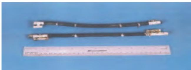
Fig. 4.7 : Bi-2223 HTS tubes of 300mm length and 10 mm diameter
