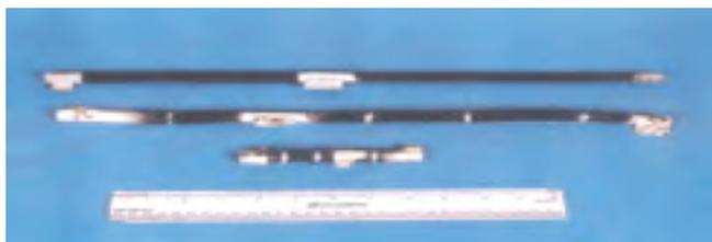
Fig. 4.8 : Low loss superconducting joints made in Bi2223 HTS tubes with  $J_c > 4500\text{A}/\text{cm}^2$  at 4.2K.
