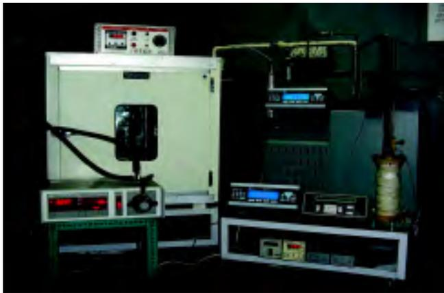
Fig. 1.8 : Two-pressure cum two-temperature RH generator
