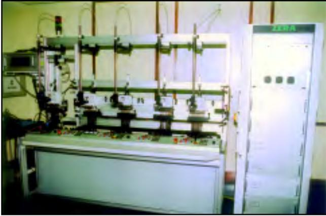
Fig. 2.10 : High accuracy electricity meter calibration bench
