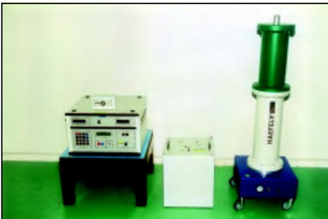
Fig. 2.11 : National Standards of AC High Voltage Ratio up to 100 kV/100 V at 50 Hz
