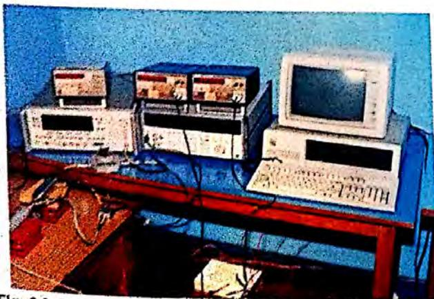
Fig. 2.8 Automated set up for comparison of high frequency thermal voltage converters used in Intercomparison
