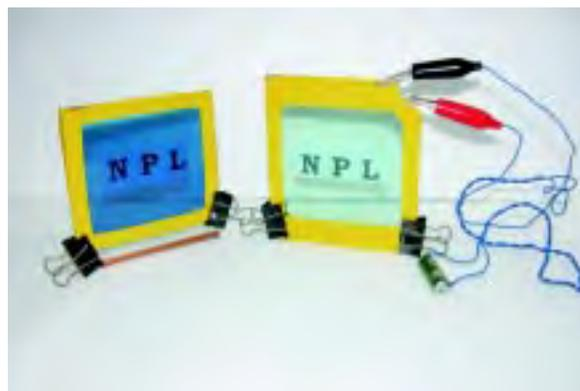
Fig. 4.9 Prototype electrochromic window developed at NPL
