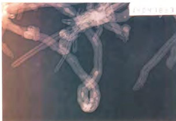
Fig. 3.7 TEM photograph of the carbon Nanotubes showing inclusion of the presence of metal catalyst inside the cavity
