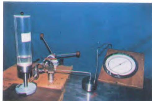
Fig.1.11 Dynamic Pressure Calibrator in operation
