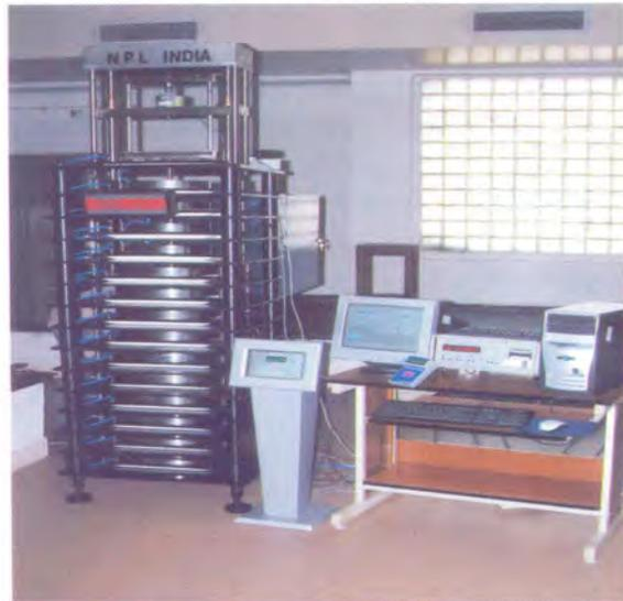
Fig. 1. 4 - Load cell testing machine
