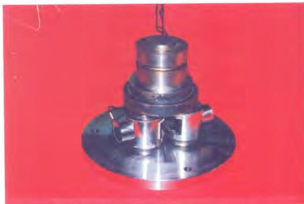
Fig. 1.1 Force transfer standard for the medium range
