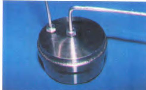
Fig. 1.9: Dynamic Pressure Calibration Chamber
