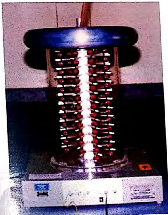
Fig. 2.4 High voltage standard resistive divider
