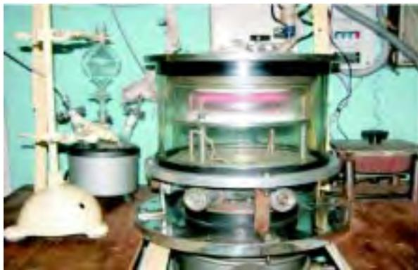
Fig. 4.7 Home-made plasma polymerization deposition system
