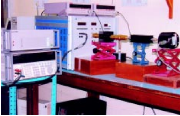
Fig. 2.1 : Set up for comparison of 30 A shunt against 20 A shunt.
