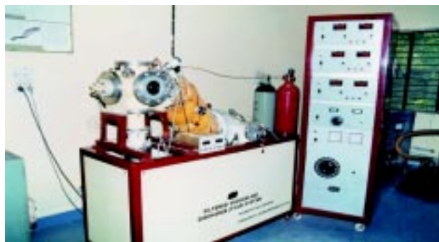
Fig. 4.3. A custom designed and indigenously developed S bend FCVA process equipment
