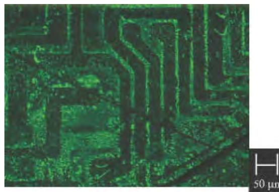
**Fig. 3.19:** Fluorescence micrographs of selectively deposited BSA\_FITC conjugated molecules on HDT coated regions.
