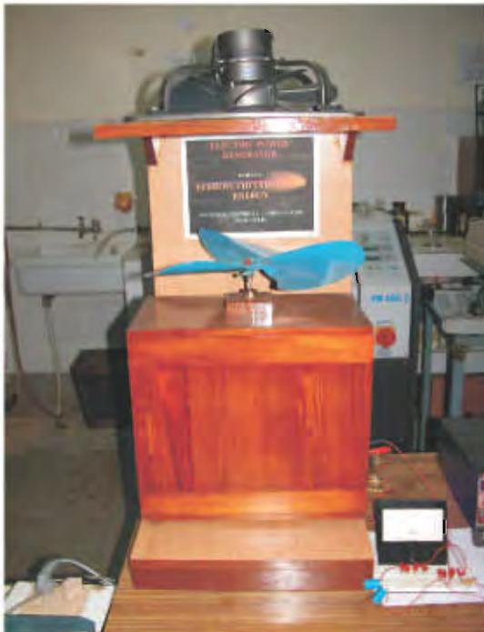
**Fig. 5.6 :** Laboratory model of a ferro-fluid based electric power generator.
