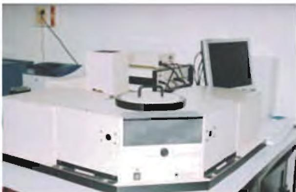
Fig. 4.1 : Combined steady state Fluorescence and Phosphorescence lifetime spectrometer.
