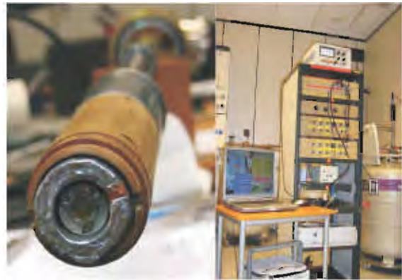
Fig. 2.3: The CCC torus with DC SQUID in the center (left Fig.) and the complete CCC-bridge with full electronics. From top of the rack: EM N11 nano-voltmeter, windings box, compensation arrangement, two double current sources, optical isolator, transmitter (VFC) and receiver (FVC). The CCC dipped in the L-He and the three multiply shielded cables carry the winding out put wired to the winding box are also seen. The SQUID electronics (MAGNICON, XXF-1) is connected to the top of the probe.
