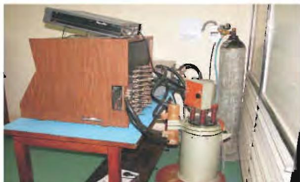
**Fig. 2.9:** Set up for shunt resistance measurement at high current
