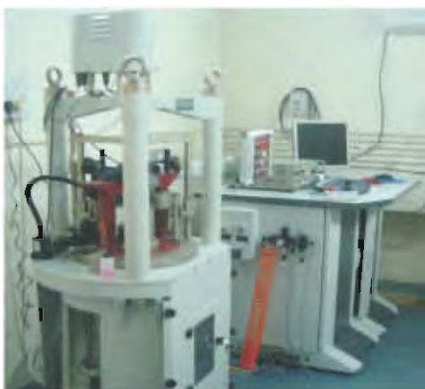
**Fig. 1.5:** Vickers cum Rockwell superficial Hardness standardizing Machine recently established
