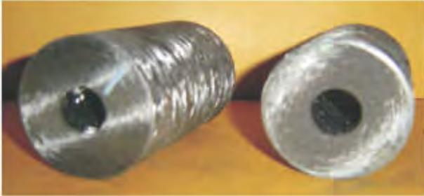
Fig. 3.6: T-300 Carbon fiber based composite tubes after carbonization
