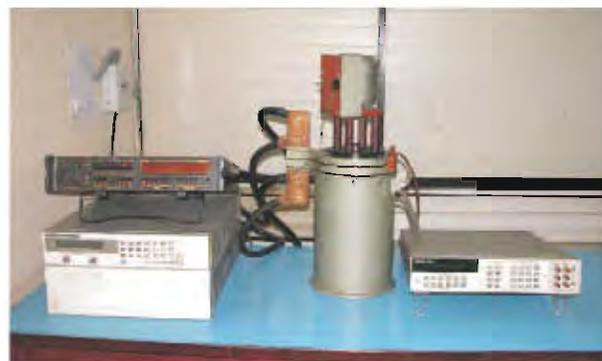
**Fig. 2.10:** Set-up for DC high Current Measurement
