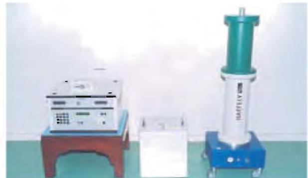
Fig. 2.12 : National Standard of AC High Voltage Ratio
