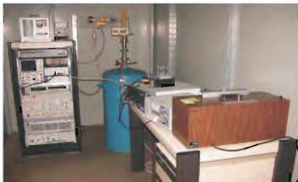
**Fig. 2.6 :** Experimental setup of Josephson series array voltage standard at 10 V level.
