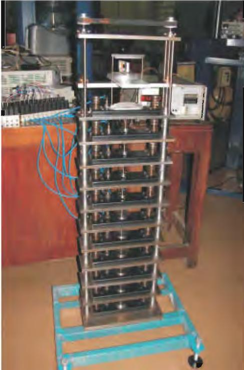
**Fig. 1.3 :** Dead weight force machine (5-50 N)
