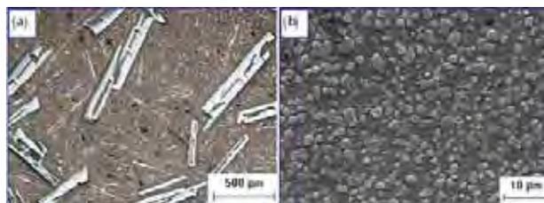
**Fig. 3.3 :** Microstructures of hypereutectic Al-30%Si (a) cast mother alloy and (b) Spray-formed alloy showing fine primary Si grains
