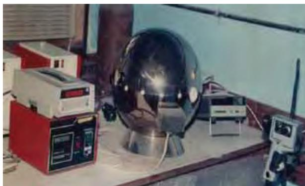
Fig. 1.2 (b) : Calibration set-up for infra-red radiation thermometers, range 50-1200 °C
