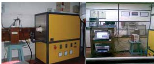
Fig. 1.2 (a) : Measurement setup and automation in thermocouple calibration, range 0-1600 °C
