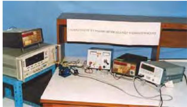
**Fig. 2.8 :** Direct Comparison Measurement Setup
