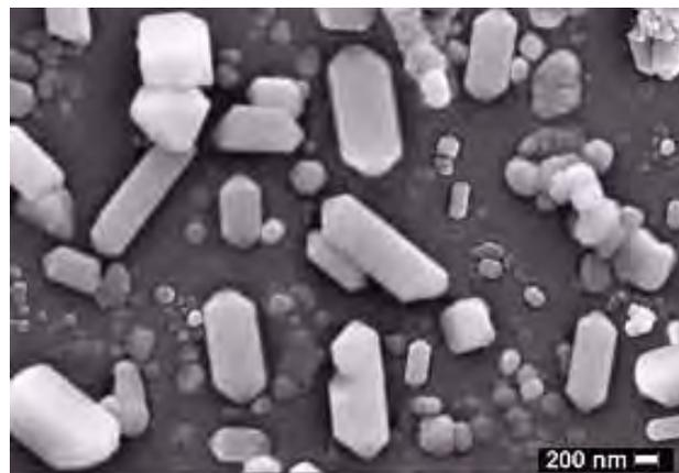
**Fig. 4.13 :** SEM micrograph of as-deposited brookite titania crystals, deposited by PECVD at - 250 V applied bias, at room temperature.
