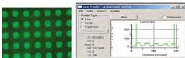
**Fig. 3.11 :** shows the two-dimensional patterning of BSA\_FITC molecules using direct μCP on glass substrate along with the intensity profiling
