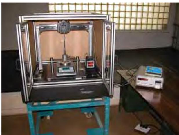
Fig. 1.5 : Low force measuring system
