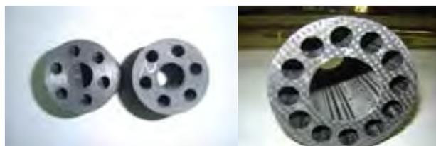
**Fig. 3.7 :** Densified C/C composite tubes samples with holes
