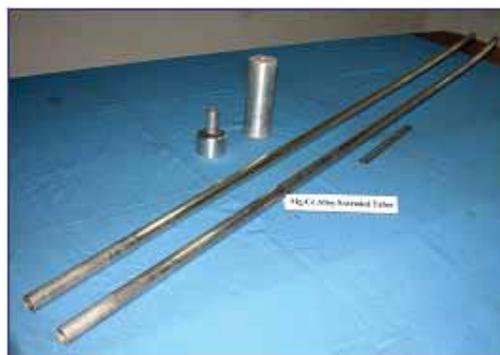
Fig. 3.2 : Mg-RE alloy extruded tubes
