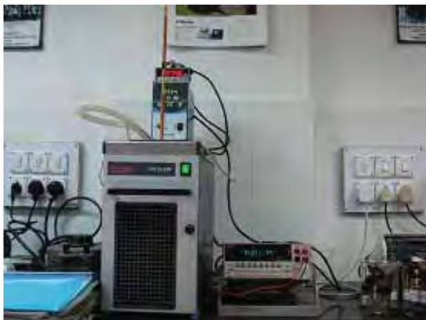
**Fig. 5.3 :** Experimental set up for ferrofluid based thermometer
