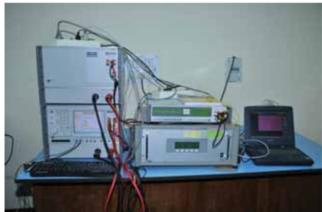
**Fig. 2.4 :** Setup for calibration of high precision reference power standards and wattconverters, using Fluke 6100A Electrical Power standard and Fluke 8½ digit Reference multimeter (8508A).
