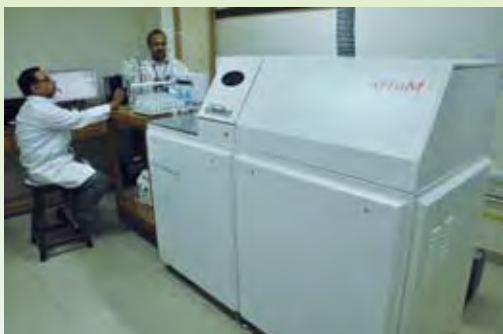
Fig. 7.18 Trace elemental analysis unity ICP-HRMS system
