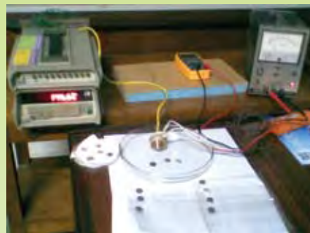
Fig.7.8 Photographs of K-Value probes with some samples.
