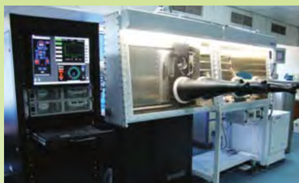
Fig. 1.2 : Glove box integrated with thermal evaporator.
