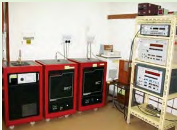
Fig. 5.5 Set-up for Realization of Fixed Point by SPRTs
