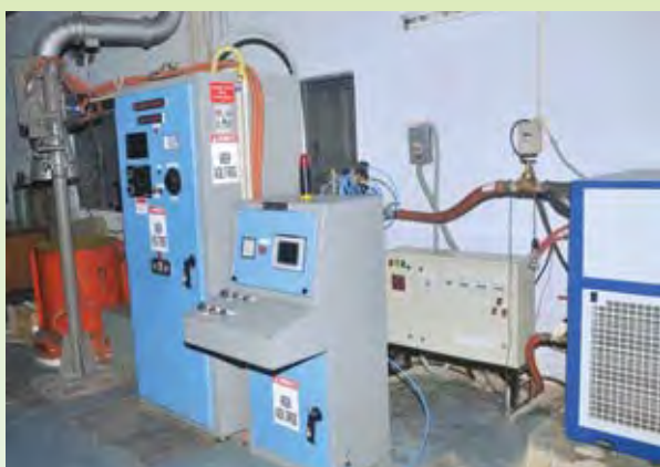
Fig. 2.23 A view of the Induction heating furnace commissioned at NPL
