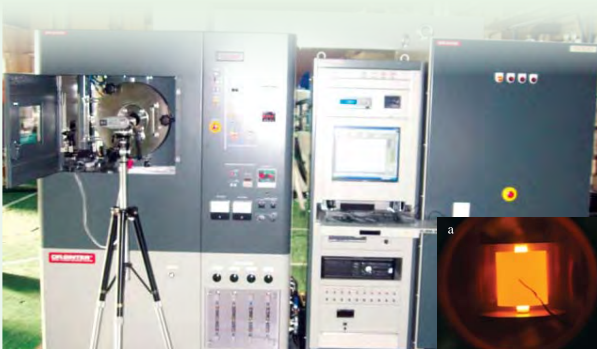
Fig. 2.46 Spark Plasma Sintering Unit (SPS) and (a) inset showing the die in hot condition during SPS
