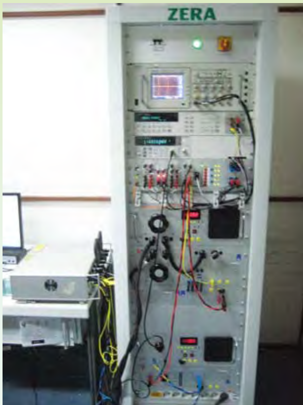
Fig. 4.14 Front side showing integrated primary standard
