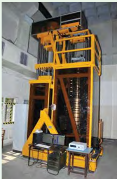
Fig. 5.9 A view of 1 MN Force Standard Machine
