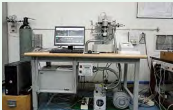
Fig. 5.12 Force Balance Piston Gauge with support equipments
