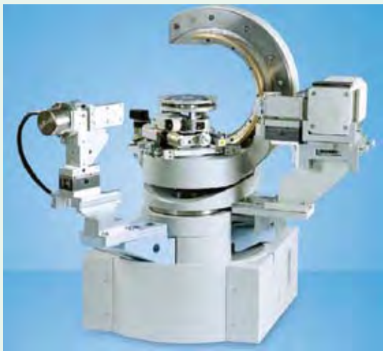
Fig. 7.5 X'Pert PRO MRD PANalytical HRXRD cum XRR system
