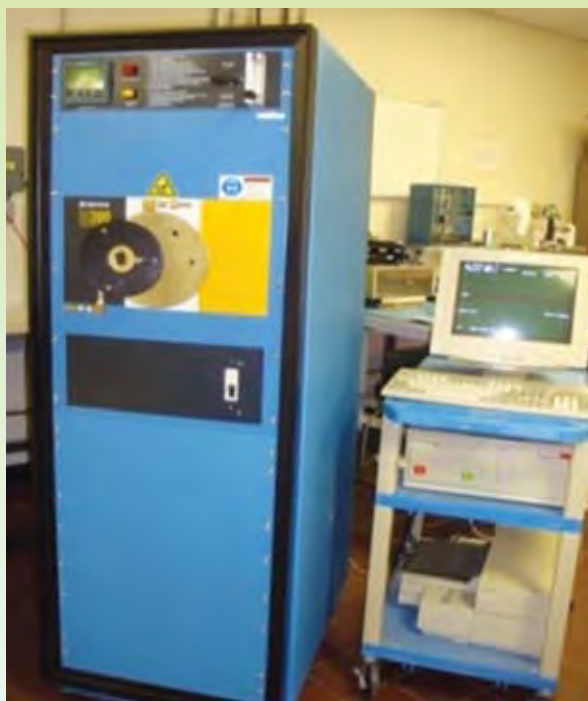
Fig. 5.6 High Temperature Blackbody Source (600-3000°C)
