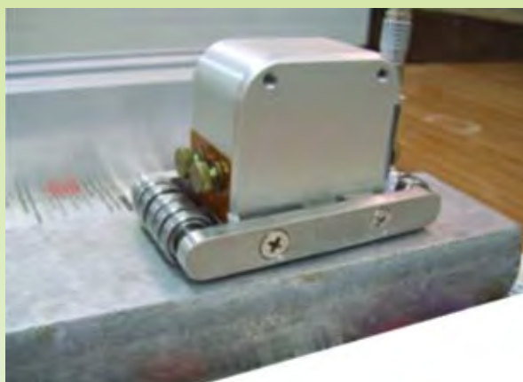
Fig. 5.23 EMAT transducer on an aluminium block
