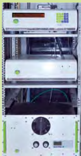
Fig. 7.15 NO, NO 2 and NO x analyzer system (Model: CLD 8xx, Make: ECO PHYSICS)
