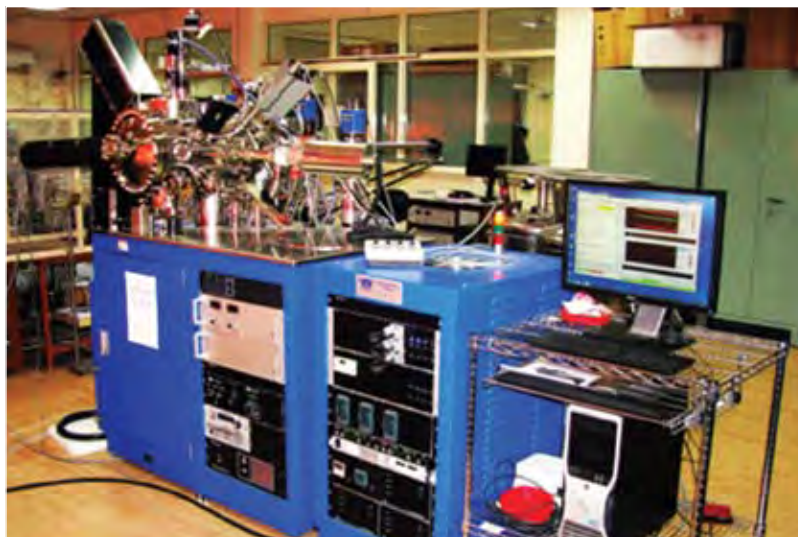
Fig. 1.33: Ultra High Vacuum Pulsed Laser Deposition (UHV-PLD) System for growth of III-Nitrides
