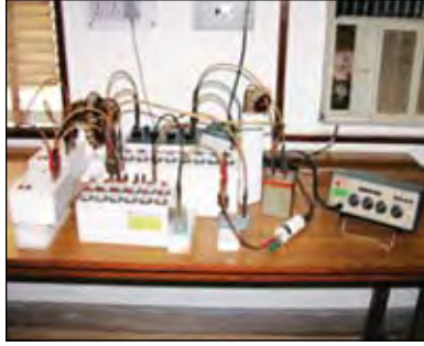
Fig. 5.13 Calibration set-up for high value capacitance standards
