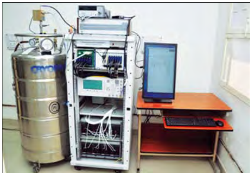
Fig. 6.1 : Photograph of the 'Programmable Josephson Voltage Standard' (PJVS) at 10 Volt at NPL-India
