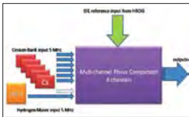
Fig. 4.12. The schematic of the alternate clock inter-comparison system using Phase Comparator. HROG is a micro phase stepper.
