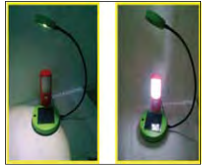
Glowing solar lamp with Li-ion battery prepared from NPL anode and CECRI cathode
