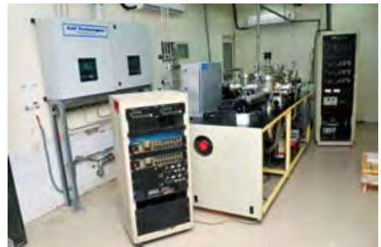
Revived a non functional 25 years old multi-chamber PECVD system (M/s GSI, USA)
