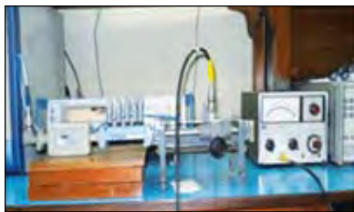
Fig. 5.19 Evaluating an adapter for its S-parameters
