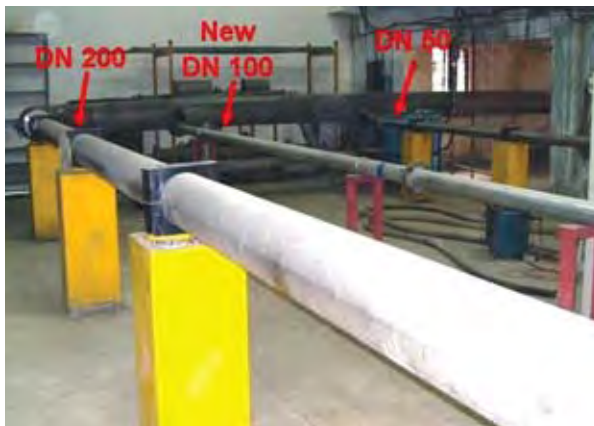
New DN100 Rig along with DN50 and DN200
