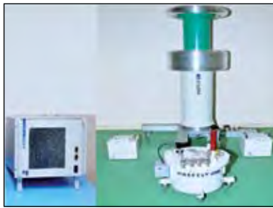
Fig. 5.23 National Standard for AC High Voltage Capacitance and Tan \delta
