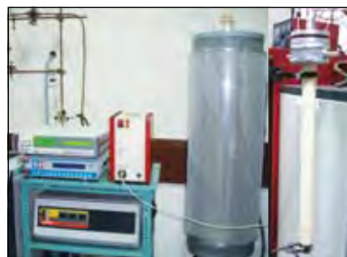
Fig. 5.25 Fixed Point Cell assembly and the Measurement Equipment for Metal-carbon Eutectic
