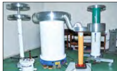
Fig. 5.21 The National Standard of AC High Current Ratio Measuring System up to 5000A/1A, 5A
