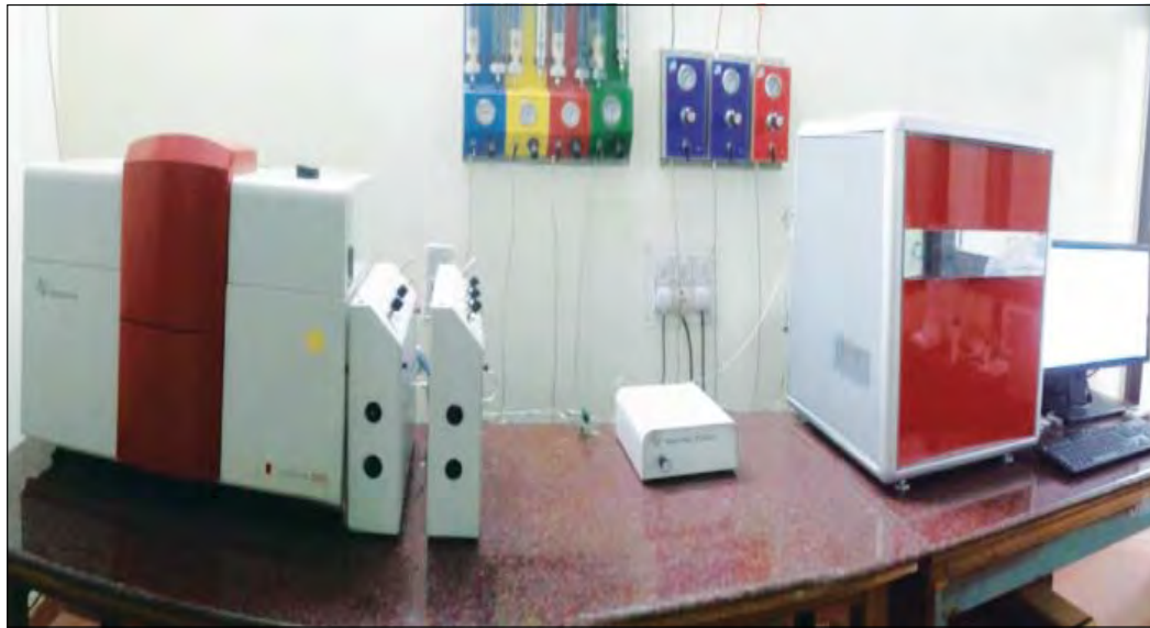
Fig. 3.20: Pyro-Cube (Elemental Analyzer) coupled with Isoprime 100 Stable isotope mass-spectrometer installed in Room no. 108 of RASD.
