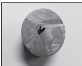
Fig. 5.3 Silicon sphere after cutting for property analysis
