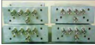
Fig. 5.14 Simulated high value inductors of 100 H, 1 kH, 10 kH and 100 kH
