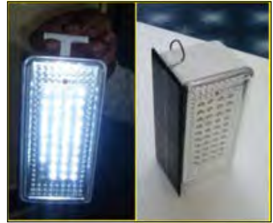
Glowing solar lantern with Li-ion battery prepared from NPL anode and CECRI cathode
