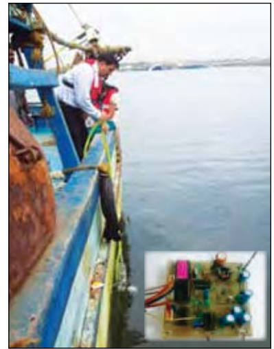
Fig. 5.44 Developed Circuit for underwater object detection and its testing at Chennai.
