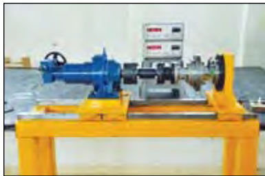
Fig. 5.9(a) Torque comparator machine using flexible coupling
