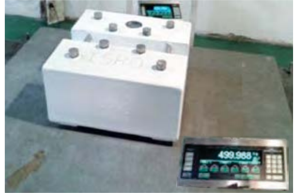
Measurement of 500 kg weight using substitution method (ABBA cycles) carried out at CSIR - NPL
