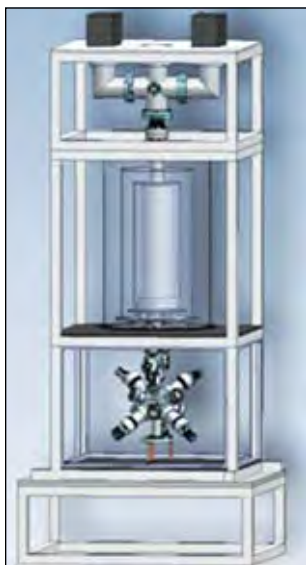
Fig. 4.4: Planned layout of the Physics package and the optical set-up of the second fountain at NPLI.
