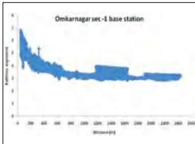
Fig 3.2. Variation of path loss exponent with distance for OM-1 base station (1800 MHz).
