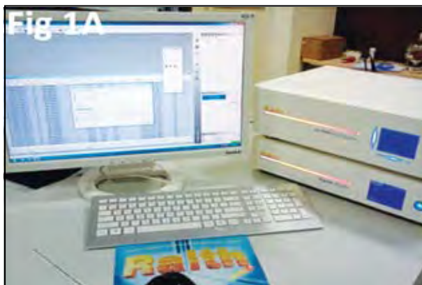
Fig 6.2a. Facility for the ebeam pattern writing
