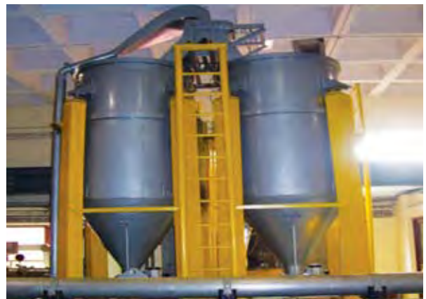
Weighing Tanks, Fishtail, Nozzle and Diverter (designed and developed in NPL)
