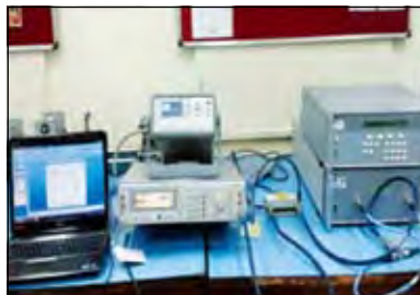
Fig. 5.17 Automated Attenuation Measurement
