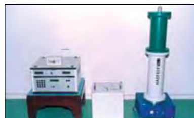
Fig. 5.22 The National Standard of AC High Voltage Ratio up to 100kV/100V comprising of the Compressed Gas Capacitor, Air Capacitor & the Electronic Voltage Divider (EVD)
