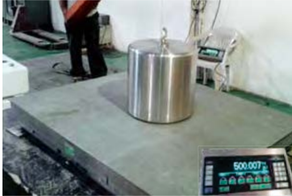
Measurement of 500 kg weight using substitution method (ABBA cycles) carried out at CSIR - NPL
