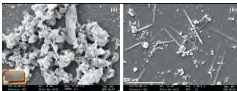
Fig. 2.11 Scanning electron micrographs of uncured (a) PPy (b) PCP3 sheet whereas inset to Figure 2.11(b) is a photograph of polypyrrole sheet
